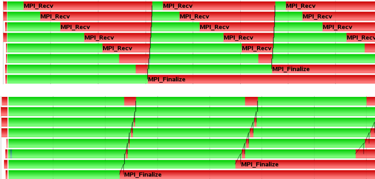
Figure 4. Vampir traces for the implementation \mathcal{P}_{mo} with (N_{pr}, N_{it}) = (8, 3) for two different load balancing strategies. Top: Vampir trace for LB1. The Parareal runtime is R_{pa} = 7.964 s. Bottom: Vampir trace for LB2. The Parareal runtime is R_{pa} = 5.436 s.
