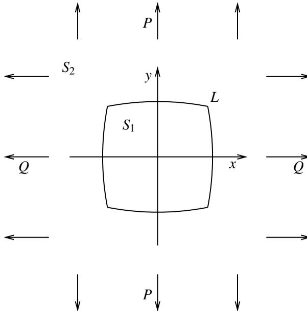
**Figure 1.** An infinite plate with a traction-free hole under uniform stresses. The cases  $P = Q$  and  $P = -Q$  correspond to remote bulk and shear, respectively. The piecewise smooth boundary of the hole has a certain rotational symmetry and possibly a finite number of corners.
