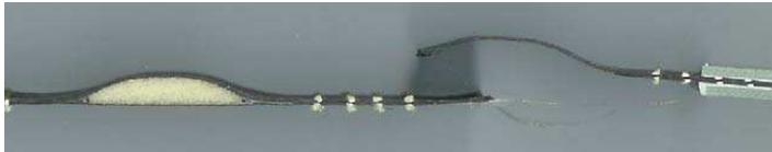
Iteration 6, T300 carbon, small circular core, with core wrapped.
