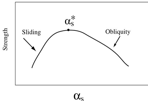
**Figure 1.** Staple yarn strength versus surface helix angle. Optimal helix angle exists due to the strengthening effects of yarn pressure and interfiber friction, and to the weakening effects of fiber obliquity as the surface helix angle is increased.
