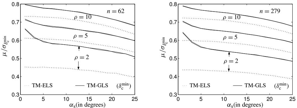
**Figure 12.** Normalized mean,  $\mu/\sigma_{\delta_c^{\min}}$ , versus surface helix angle,  $\alpha_s$ . The TM-GLS results are for  $f = 0.1$  and  $0.3$ . TM-ELS results are from [Porwal et al. 2006].
