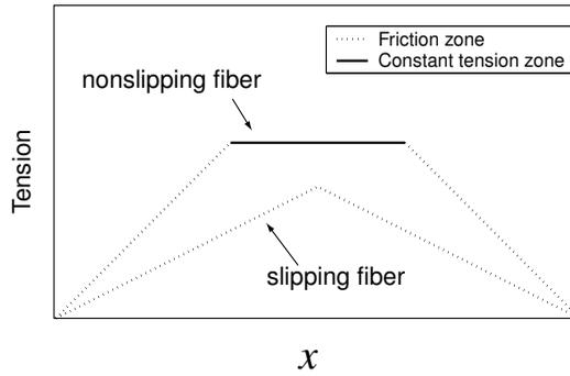
**Figure 4.** Tensile stress profiles in the fibers.
