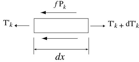
**Figure 3.** Development of tension in the fiber near a break in layer  $k$ .
