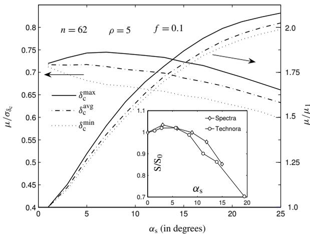
**Figure 14.** Normalized mean bundle strength  $\mu / \sigma_{\delta_c}$  and  $\mu / \mu_1$  versus surface helix angle  $\alpha_s$  for different length scales. Here  $\mu_1$  is the value at  $\alpha_s = 1^\circ$ . Inset figure ( $S/S_0$  versus  $\alpha_s$ ) is plotted using data from [Rao and Farris 2000], where  $S_0$  is the yarn strength when  $\alpha_s = 0^\circ$ .
