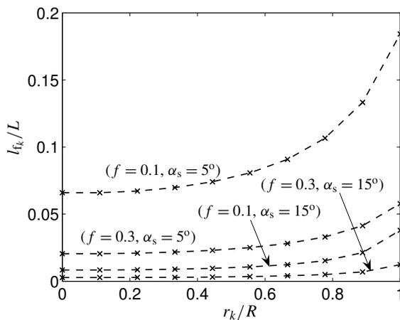
**Figure 8.** Normalized friction length,  $l_k/L$ , versus normalized yarn radius,  $r_k/R$ . Here  $l = 10$  and  $n = 279$ .
