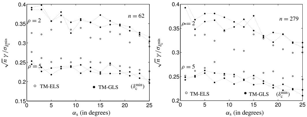
**Figure 13.** Normalized standard deviation  $\sqrt{n} \gamma / \sigma_{\delta_c^{\min}}$  versus surface helix angle  $\alpha_s$ . The TM-GLS results are for  $f = 0.1$  and  $0.3$ . TM-ELS results are from [Porwal et al. 2006].
