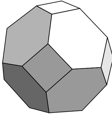
**Figure 1.** Open cell, Kelvin form, truncated octahedron.
