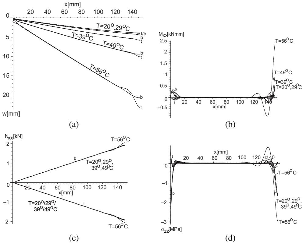
**Figure 7.** Nonlinear response along sandwich panel loaded simultaneously by a mechanical load and thermally induced deformations with a zero thermal gradient at various temperatures: (a) vertical displacements, (b) bending moments, (c) in-plane stress resultants, (d) interfacial vertical normal stresses at interfaces. Legend: — t upper face/ interface; - - - b lower face/interface.
