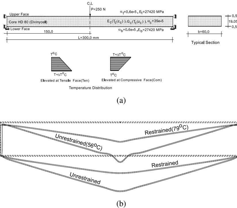
**Figure 6.** Geometry and deformed shapes of sandwich panel loaded by a mechanical load and thermally induced deformations with a zero thermal gradient: (a) geometry of unrestrained and restrained panels; (b) deformed shape of an unrestrained at  $T = 56^{\circ} C$  and a restrained panel at  $T = 79^{\circ} C$ .
