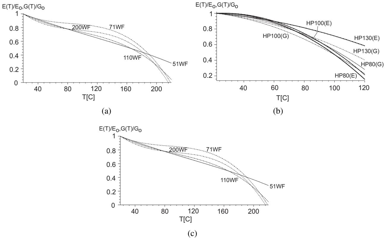
**Figure 2.** Normalized temperature-dependent elastic and shear moduli of various poly-mer foam cores: (a) Rohacell WF foam, (b) Divinycell HP foam, (c) Divinycell P foam. Legend: (E) – modulus of elasticity (thick lines), (G) – Shear modulus (dashed thin lines).
