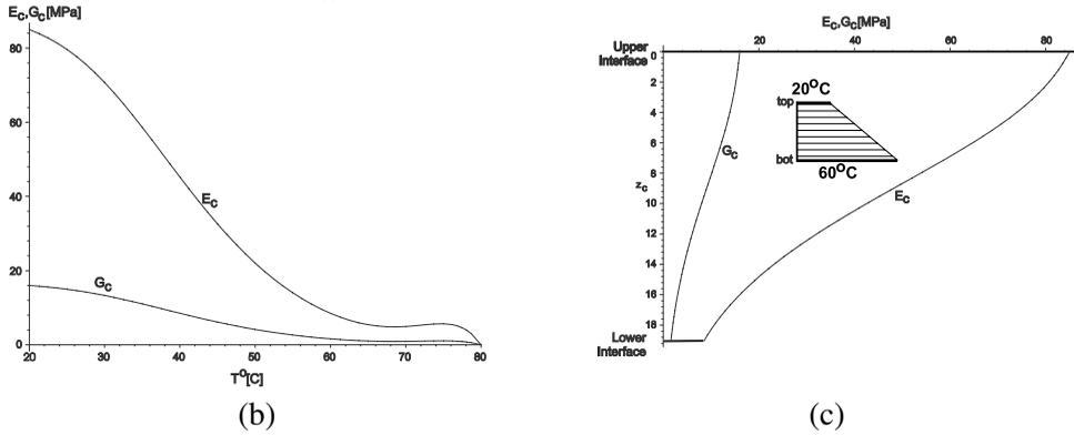
**Figure 3.** Geometry and temperature-dependent properties of the core and its distribution: (a) geometry and mechanical properties; (b) temperature dependence of elastic and shear moduli of core; (c) distribution of moduli through depth of core for a thermal gradient of 40° C
