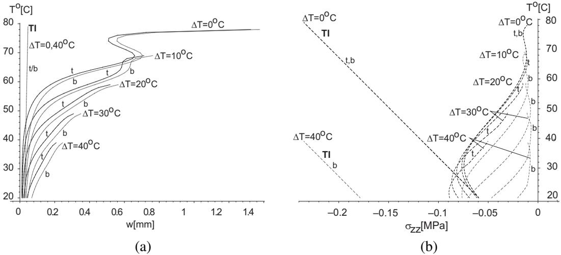
**Figure 5.** Temperature equilibrium curves of maximum values for a restrained sandwich panel subjected to various thermal gradients: (a) maximum vertical displacements of face sheets, (b) maximum compressive interfacial vertical normal stresses at interfaces. Legend: — t upper face or interface; - - - b lower face or interface.
