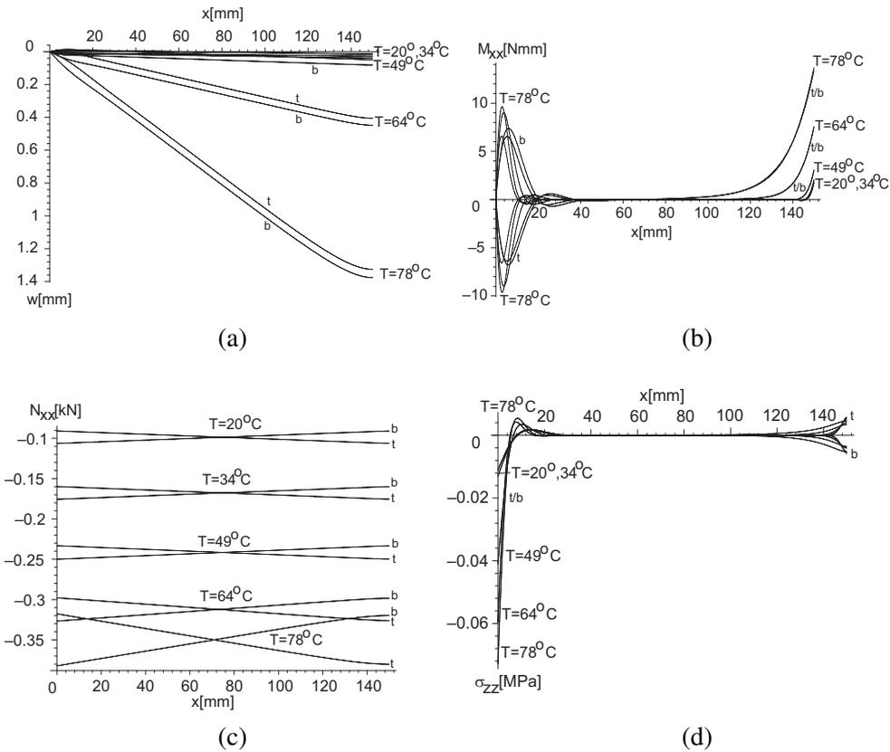
**Figure 4.** Postbuckling results along the length of a restrained sandwich panel with a zero thermal gradient at various temperatures: (a) vertical displacements, (b) bending moments, (c) in-plane stress resultants, (d) interfacial vertical normal stresses at interfaces. Legend: — t upper face/ interface; - - - b lower face/ interface.
