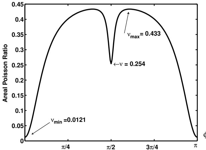
**Figure 2.** Areal Poisson’s ratio for graphite (hexagonal).
