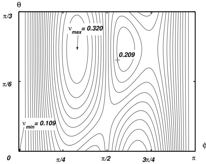
Figure 6. Areal Poisson's ratio for MgSiO<sub>3</sub> ilmenite.
