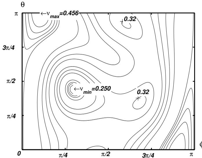
Figure 9. Areal Poisson's ratio for copper sulphate pentahydrate.
