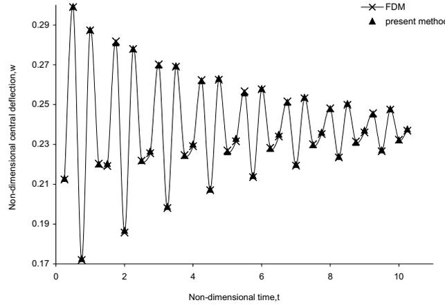
**Figure 8.** Damped response of a simple supported banana fiber reinforced square orthotropic plate for  $C_v = 1.25$ .
