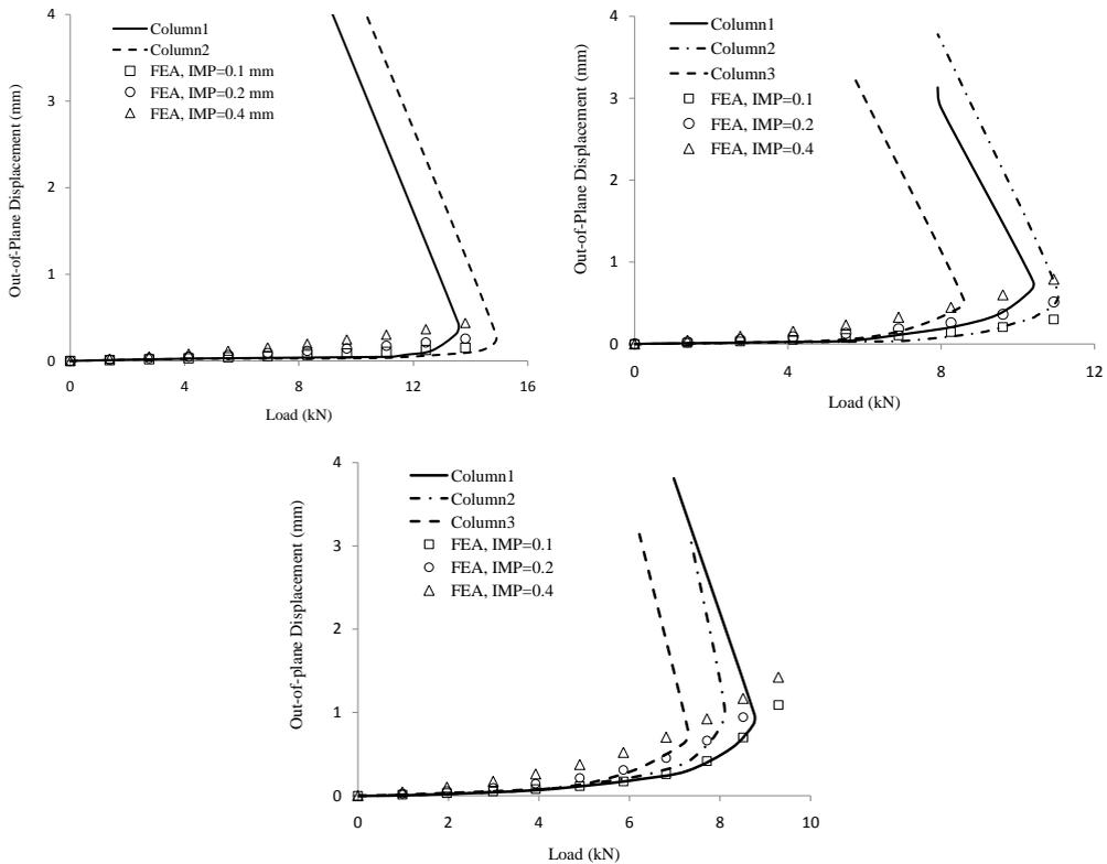
**Figure 16.** Finite element and experimental results for out-of-plane versus load diagram for columns with H100 core and (a) 25.4 mm debond, (b) 38.1 mm debond, (c) 50.8 mm debond. The average initial imperfection magnitude in the tested columns is 0.2 mm.
