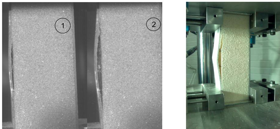
**Figure 6.** Left: High speed images showing the debond in a column with H45 core and 50.8 mm debond length 1 ms before propagation (1) and right after propagation has taken place (2). Right: Crack kinking into the core in a column with H100 core and 25.4 mm debond length.
