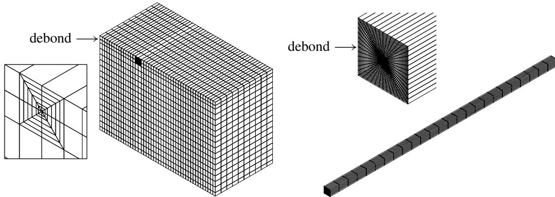
**Figure 14.** Finite element models. Left: half-model showing the mesh in the global model. The smallest element size is 0.2 mm. Right: submodel showing the refined mesh. Element size close to the crack tip is 10  $\mu\text{m}$ .
