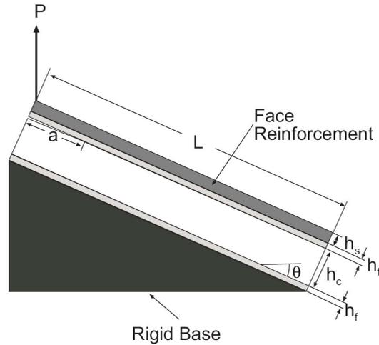
**Figure 8.** Schematic representation of the modified TSD specimen.
