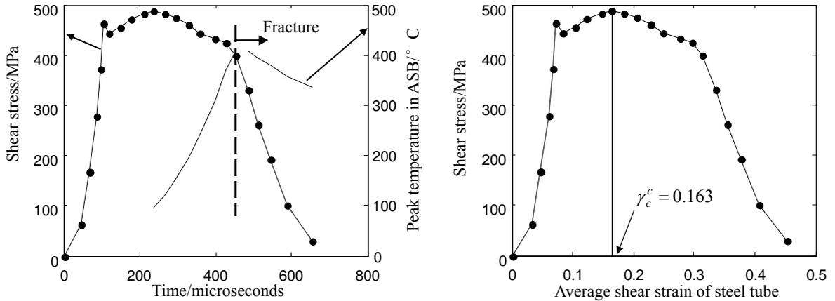
**Figure 4.** Left: Experimentally observed curves of shear stress and ASB peak temperature versus time. From [Hartley et al. 1987]. Right: Shear stress versus average shear strain curve for a steel tube, based on values on the left.
