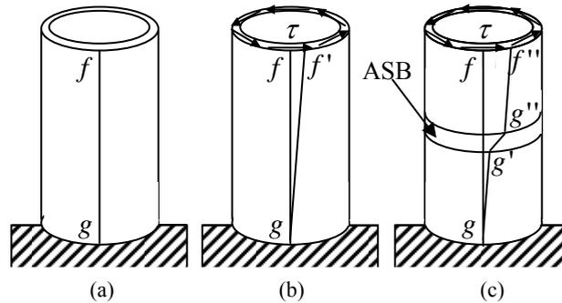
**Figure 2.** A thin-walled tube specimen without deformation (a), the uniform shear deformation in the elastic and strain-softening stages (b), and the localised shear deformation in the ASB and uniform shear deformation outside the ASB (c).
