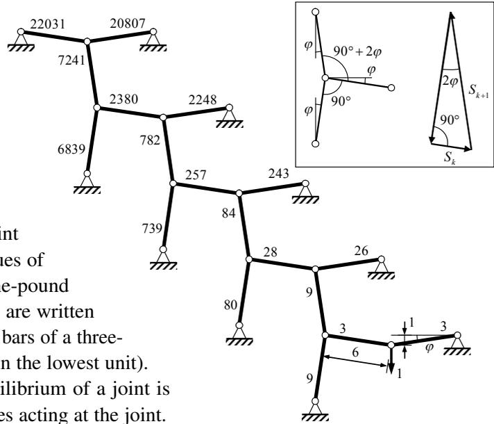
**Figure 6.** The inextensional bar-and-joint model of Leonardo’s structure. The values of the forces in the bars, arising from a one-pound vertical load at the lowest internal joint, are written on the respective bars. Forces in the two bars of a three-pinned frame unit are different (except in the lowest unit). In the upper right-hand corner, the equilibrium of a joint is shown by the vector triangle of bar forces acting at the joint.
