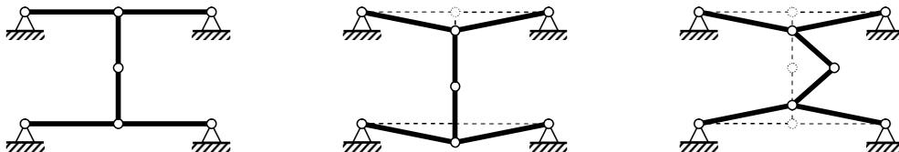
**Figure 1.** A two-DOF infinitesimal mechanism in the plane. Left: initial state. Middle: a displacement where the horizontal bars undergo second-order elongation. Right: a displacement where the same bars undergo fourth-order elongation.
