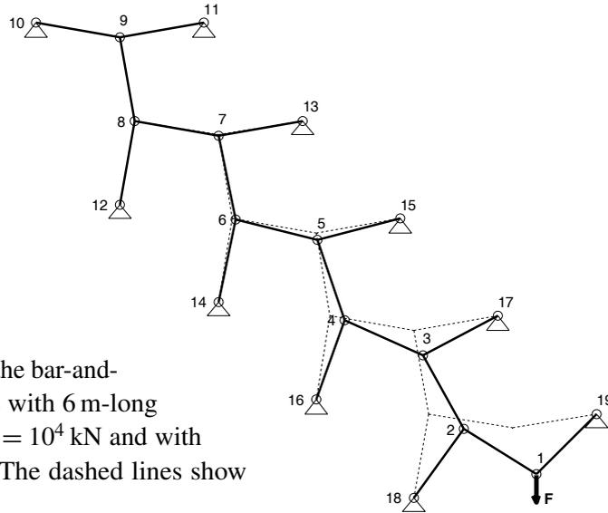
**Figure 7.** The equilibrium shape of the bar-and-joint model of Leonardo's structure with 6 m-long linearly elastic bars of stiffness  $EA = 10^4$  kN and with a vertical load  $F = 1$  N at joint 1. The dashed lines show the structure at the rest position.
