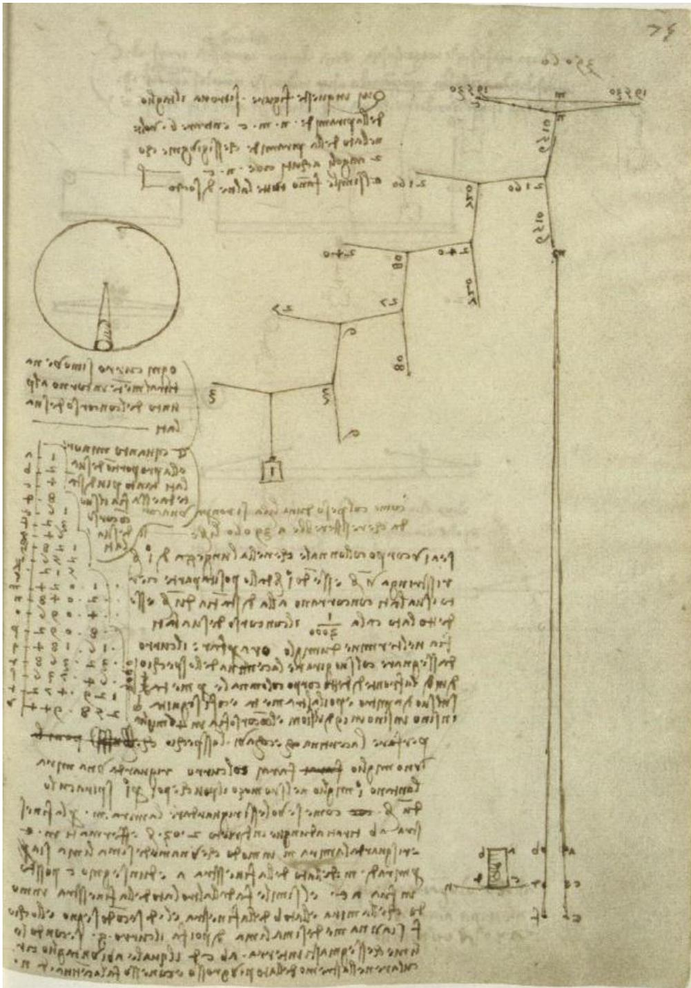
**Figure 5.** Leonardo da Vinci's drawing of a planar assembly [Leonardo 1493, folio 75R]. The forces in the cables, arising from a one-pound load at the lowest cable, are written on the respective cables. Leonardo, as usual, made this note in mirror image.
