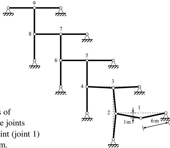
**Figure 4.** A chain-like planar assembly composed of nine three-pinned frame units of collinear joints, and displacements of middle joints (numbered 1 through 9) when the lowest joint (joint 1) has a prescribed vertical displacement of 1 m.
