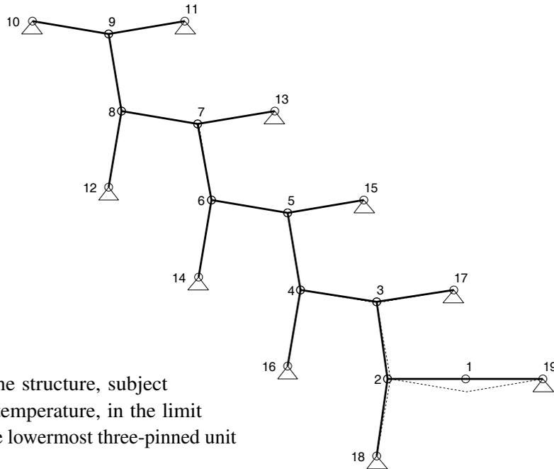
**Figure 8.** The shape of the structure, subject to a uniform decrease in temperature, in the limit state where the joints of the lowermost three-pinned unit become collinear.
