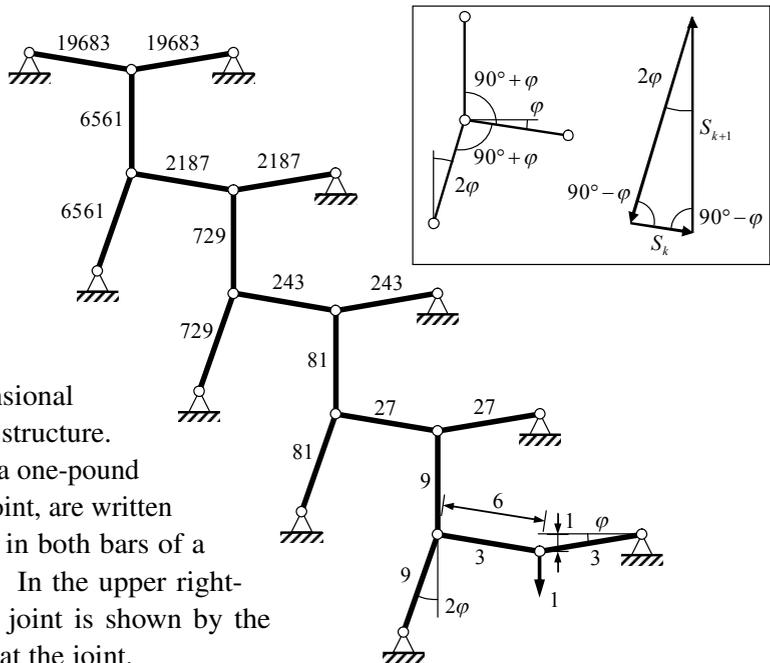
**Figure 10.** The modified inextensional bar-and-joint model of Leonardo's structure. The forces in the bars, arising from a one-pound vertical load at the lowest internal joint, are written on the respective bars. The forces in both bars of a three-pinned frame unit are equal. In the upper right-hand corner, the equilibrium of a joint is shown by the vector triangle of bar forces acting at the joint.
