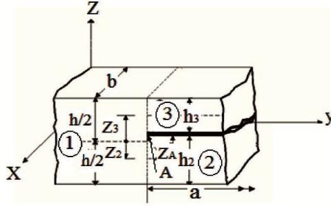
**Figure 2.** Plate elements at a delamination crack tip.
