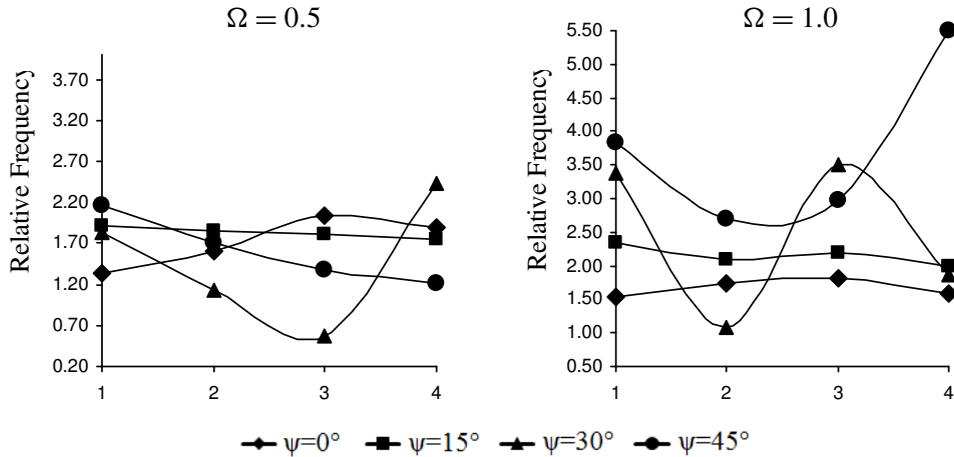
**Figure 5.** Variation of relative frequencies (NDF) of graphite-epoxy bending stiff composite conical shells with delamination at rotation speeds  $\Omega = 0.5$  (left) and  $\Omega = 1.0$  (right) for different twist angles  $\Psi$  and different numbers of delaminations. Other parameters are  $n = 8$ ,  $h = 0.0004$ ,  $a/L = 0.33$ ,  $d/L = 0.5$ ,  $s/h = 1000$ ,  $L/s = 0.7$ ,  $\theta_0 = 45^\circ$ , and  $\theta_v = 20^\circ$ .
