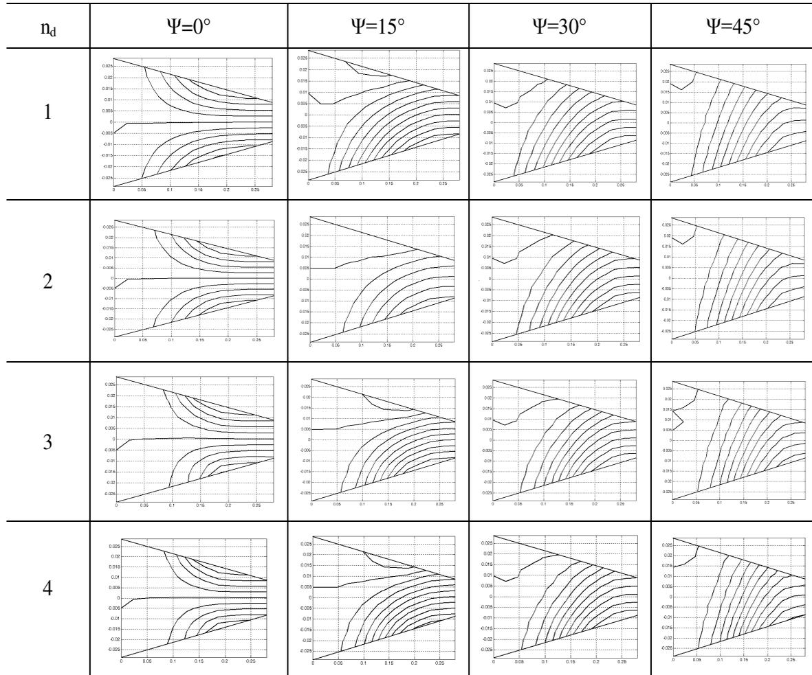
**Figure 6.** Effect of twist and number of delaminations on mode shapes for NDF of graphite-epoxy bending-stiff delaminated composite conical shells, considering  $n = 8$ ,  $h = 0.0004$ ,  $s/h = 1000$ ,  $a/L = 0.33$ ,  $d/L = 0.5$ ,  $L/s = 0.7$ ,  $\theta_0 = 45^\circ$ , and  $\theta_v = 20^\circ$ .
