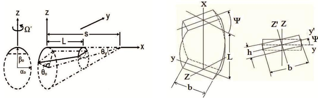
**Figure 1.** Geometry of an untwisted conical shell (left) and a twisted plate (right).
