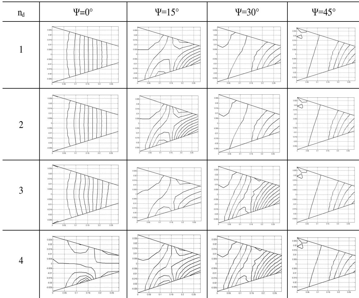
**Figure 7.** Effect of twist and number of delaminations on mode shapes for NDSF of graphite-epoxy bending-stiff delaminated composite conical shells, considering  $n = 8$ ,  $h = 0.0004$ ,  $s/h = 1000$ ,  $a/L = 0.33$ ,  $d/L = 0.5$ ,  $L/s = 0.7$ ,  $\theta_0 = 45^\circ$ , and  $\theta_v = 20^\circ$ .
