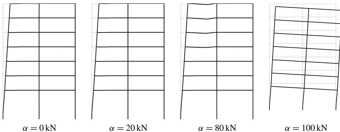
**Figure 9.** The collapse modes of the seven-story frame.
