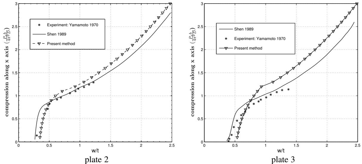
**Figure 9.** Uniaxial compression versus maximum deflection with a constant lateral pressure by the present method, the perturbation method [Shen 1989] and the experiment [Yamamoto et al. 1970]. Axial load versus deflection: plate 2 (left) and plate 3 (right).
