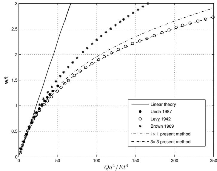
**Figure 5.** Square plate: central deflection versus lateral pressure.
