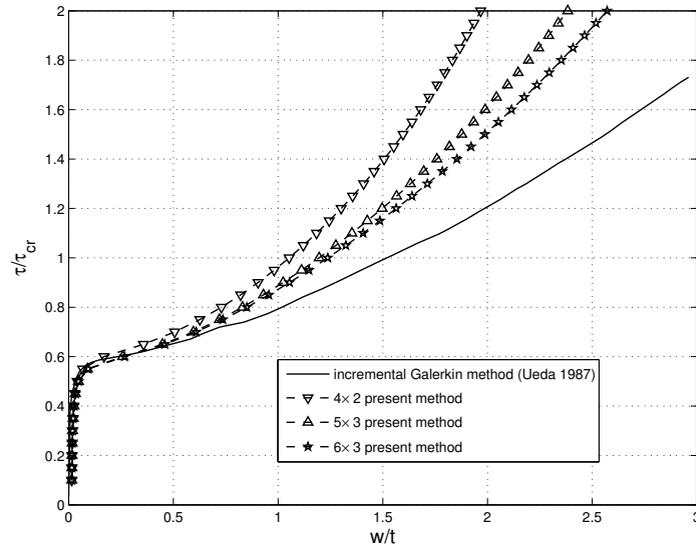
**Figure 14.** Comparisons of load-deflection curves as given by present global Galerkin method and the incremental Galerkin method [Ueda et al. 1987] under uniaxial compression combined with a shearing load.
