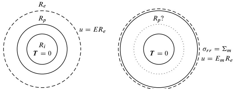
**Figure 5.** The hollow sphere. Left: the direct problem. Right; the inverse problem under given boundary conditions on  $R_e$ . On the dashed circle the displacement is prescribed, on the solid-line circle the traction is given.
