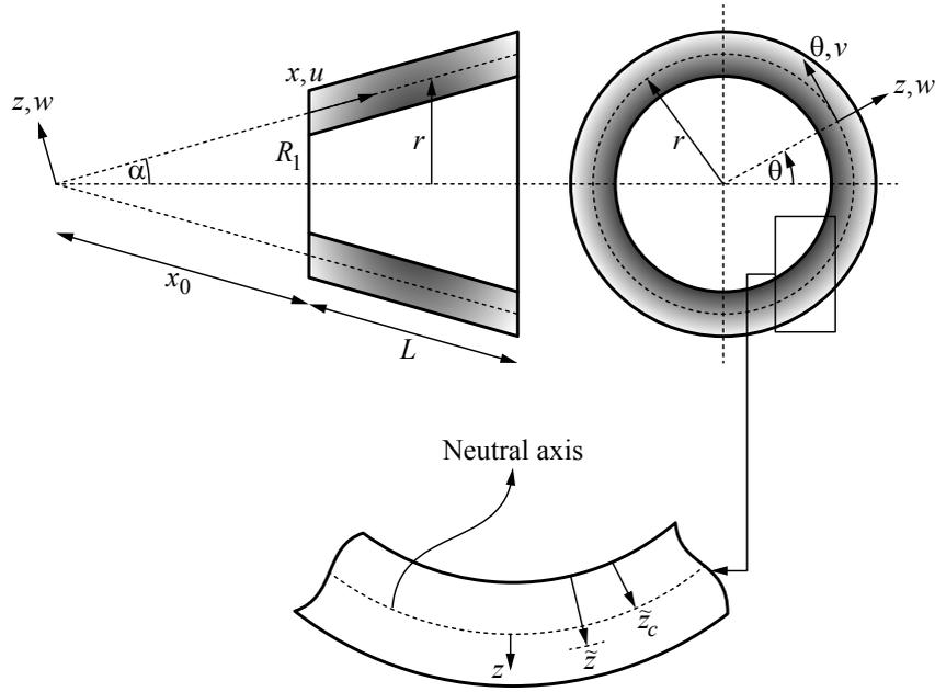
**Figure 1.** Schematic view of truncated conical shell.
