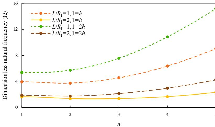
**Figure 5.** Effects of circumferential wave number and dimensionless length on dimensionless natural frequency,  $\alpha = 30^\circ$ ,  $N = 1$ .
