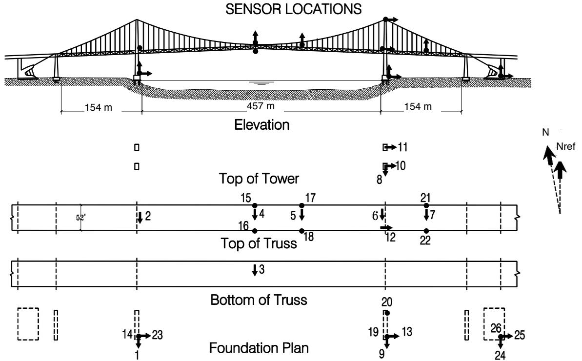
Figure 6. Sensor locations, from [Smyth et al. 2003].
