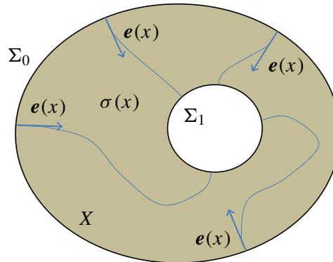
**Figure 3.** Geometry of an annulus in two space dimensions with boundaries  $\Sigma_0$  and  $\Sigma_1$ , the level sets where  $u = 0$  and  $u = 1$ , respectively. The four curves correspond to four integrals of the flow of the gradient vector field  $\widehat{\nabla}u$ .
