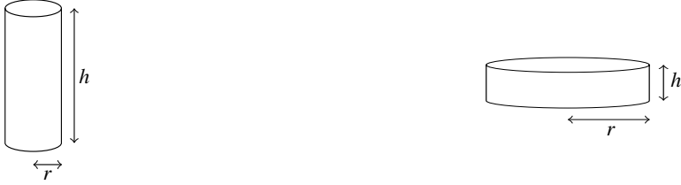
This rigid body is inertially oblong if h^2 > 6r^2 . This rigid body is inertially oblate if h^2 < 6r^2 .
