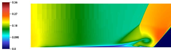
**Figure 14.** Magnification of the lambda shock-boundary layer pattern in the viscous calculation. Density (in  $\text{kg}/\text{m}^3$ ) shown here.
