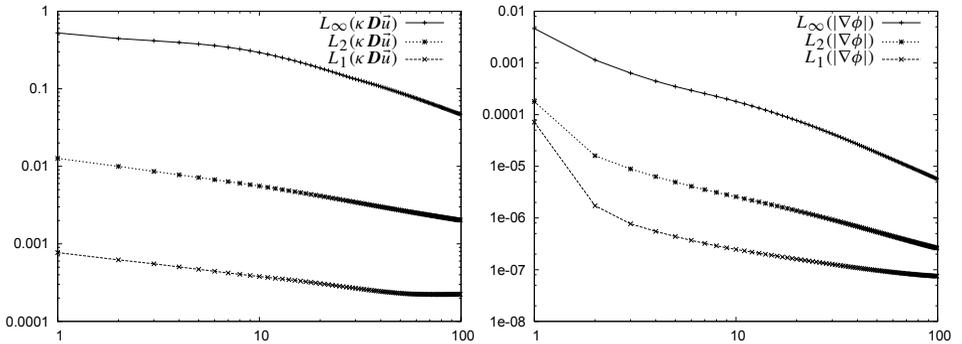
**Figure 4.** Norms ( $L_\infty$ ,  $L_2$  and  $L_1$ ) of  $\kappa \mathbf{D}\vec{u}$  (left) and  $\nabla \phi$  (right) versus the number of projection iterations in the 2D test with  $h = \frac{1}{256}$ .
