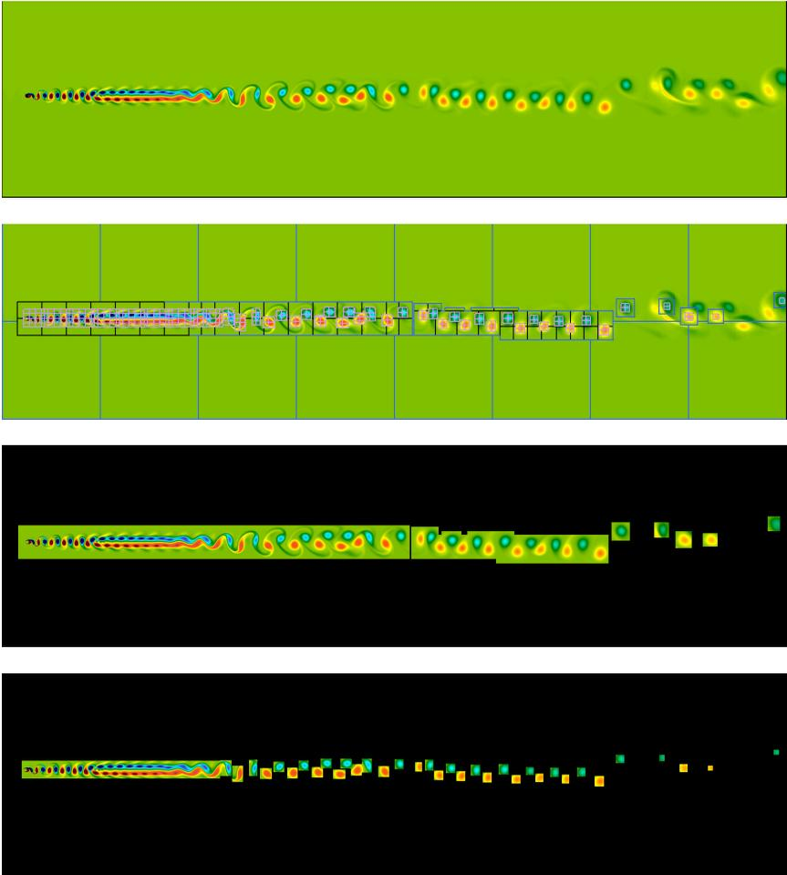
**Figure 15.** 2D flow past a cylinder at  $Re = 300$  with extended wake ( $l = 32$ ). From top to bottom: vorticity, AMR hierarchy of boxes enclosing the wake and two finest levels. The cylinder has radius  $r = 0.0625$  and is shown as a black spot near the inlet. Wake extends approximately 250 cylinder diameters. Time simulated is 112 seconds.
