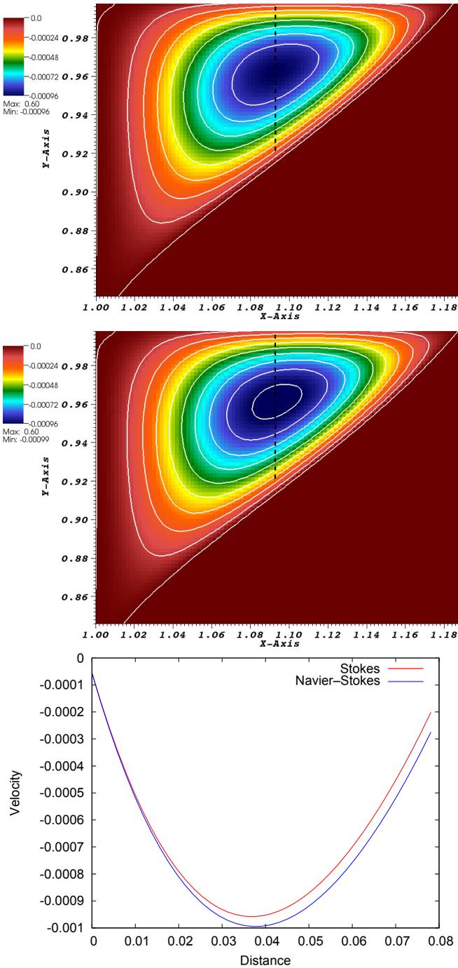
**Figure 6.** Zoomed-in view of the recirculation zone in the corner behind the backward-facing step for  $Re = 0.1$ . Top: solution to the Stokes equation. Middle: solution to the Navier–Stokes equation. Bottom: plots of velocity along the dotted lines in the top figures.
