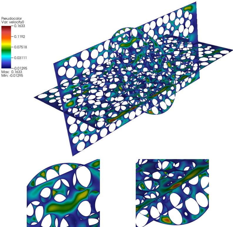
**Figure 9.** Steady-state flow through the packed cylinder geometry in Figure 7 (middle). Axial velocity is shown with magnified views of the top and bottom of the cross-sectional slice. Inlet axial velocity is 0.01 cm/sec with  $Re = 0.5$ . Computation was performed on NERSC Cray XC30 Edison using 65,536 processor cores.
