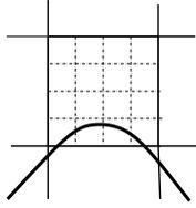
**Figure 3.** Illustration of an under-resolved geometry. When the curvature of the implicit function is too great to be resolved, we refine locally and sum the finer moments to compute the under-resolved cell's moments.
