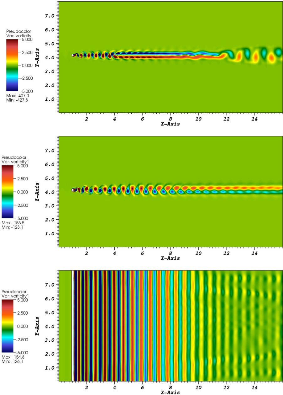
**Figure 14.** Flow past a cylinder at  $Re = 300$ . Top: 2D simulation of vorticity. Middle: 3D simulation of  $y$  vorticity in the  $x$ - $z$  plane at  $z = 4.125$ . Bottom: 3D simulation of  $y$  vorticity in the  $x$ - $y$  plane at  $y = 4$ . The cylinder has radius  $r = 0.0625$  and is shown in white centered at  $x = 1$ ,  $y = 4.125$  in 2D and  $x = 1$ ,  $y = 4$ ,  $z = 4.125$  in 3D. Time simulated is 98 seconds.
