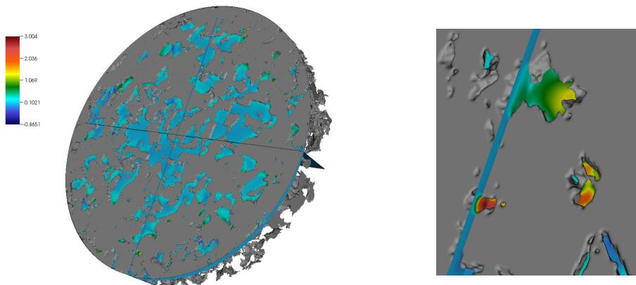
**Figure 12.** Steady-state flow through Bedford limestone: embedded boundary grid in gray with  $z$ -velocity data (left) and magnification of the bottom of the disk (right). Resolution is  $h = 43$  nm with  $2048 \times 2048 \times 320$  total grid cells and 29% porosity. Inlet velocity is  $0.0376$  cm/sec. Computation was performed on OLCF Titan using 40,960 processor cores.
