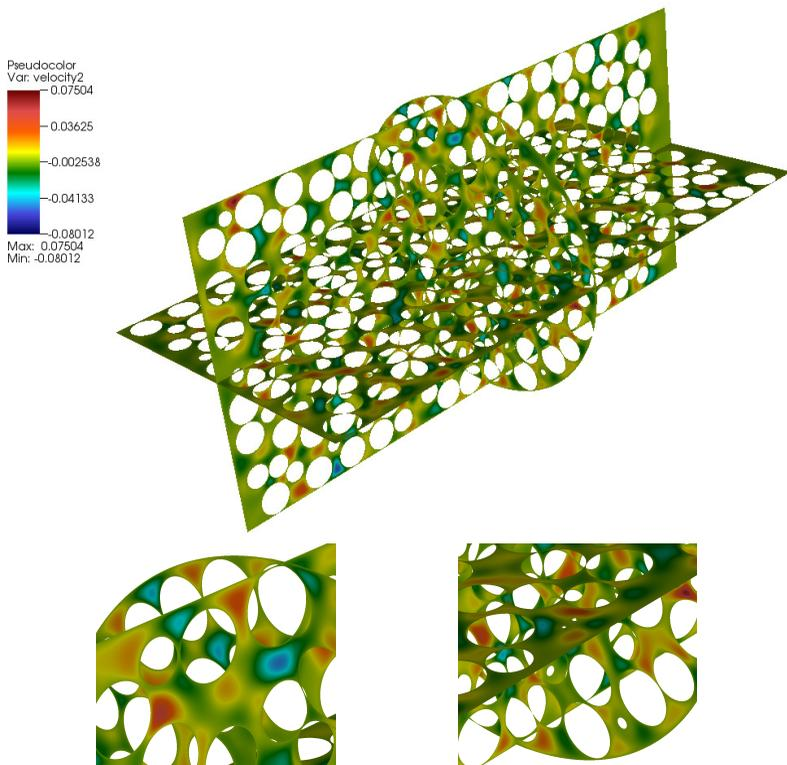
**Figure 10.** Steady-state flow through the packed cylinder geometry in [Figure 7](#) (middle). Transverse ( $z$ ) velocity shown with magnified views of the top and bottom of the cross-sectional slice. Inlet axial velocity is 0.01 cm/sec with  $Re = 0.5$ . Computation was performed on NERSC Cray XC30 Edison using 65,536 processor cores.
