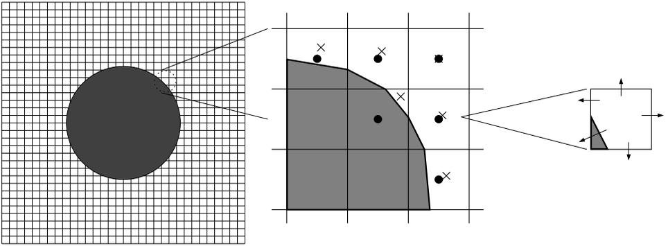
**Figure 1.** Left: example of an irregular geometry on a Cartesian grid. Middle: close-up view of embedded boundaries “cutting” regular cells. Right: single cut cell showing boundary fluxes. The shaded area represents the volume of cells excluded from the domain. Dots represent cell centers. Each “x” represents a centroid.
