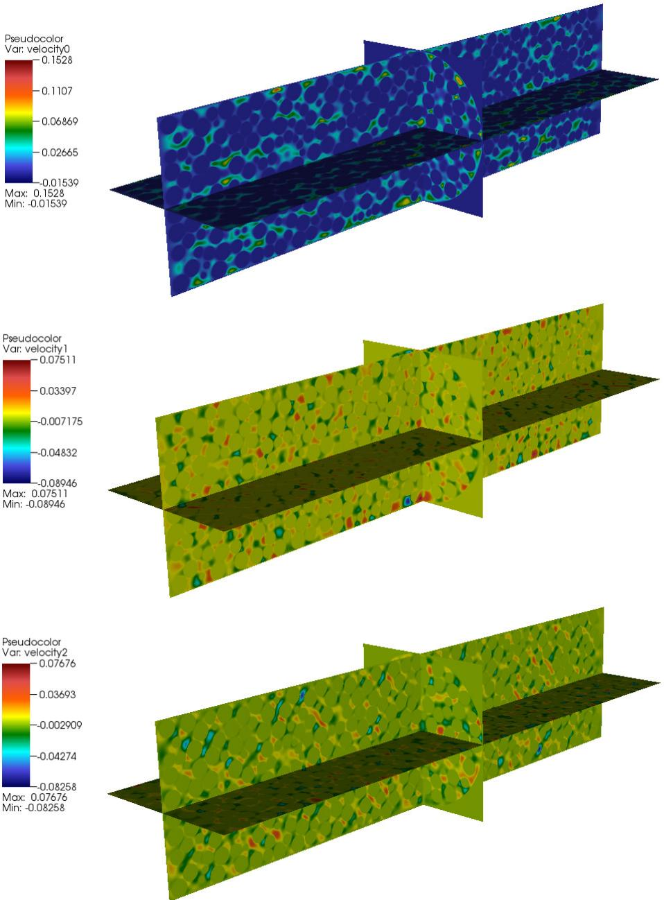
**Figure 11.** Steady-state flow through the packed cylinder geometry in Figure 7 (right). From top to bottom, we show the axial ( $x$ ) and transverse ( $y$ ) and ( $z$ ) velocities. Inlet axial velocity is 0.01 cm/sec with  $Re = 0.5$ . Spheres have not been voided in the visualization unlike in Figures 9 and 10. Computation was performed on OLCF Titan using 131,072 processor cores.
