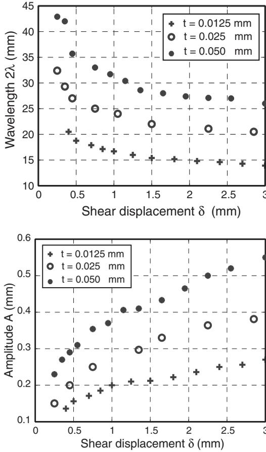
**Figure 8.** Average wrinkle wavelengths measured in the  $x$ -direction (top) and average wrinkle amplitudes (bottom) in sheared membranes of different thicknesses.
