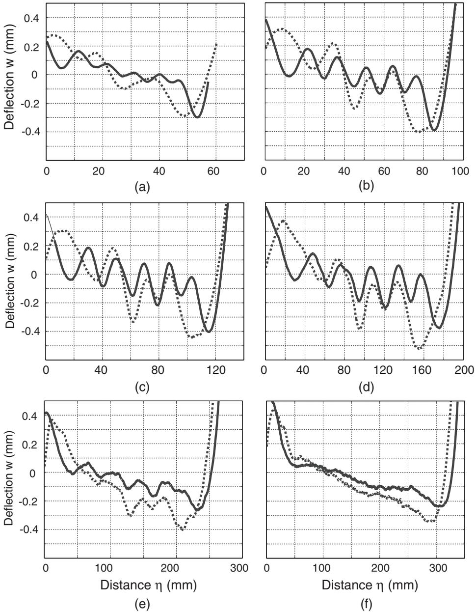
**Figure 9.** Wrinkle profiles in 0.025 mm thick, square Kapton<sup>®</sup> membrane, for  $T = T_1 = T_2 = 5$  N (dashed) and  $T = T_1 = T_2 = 20$  N (solid), at following distances from corner (a)  $\xi = 35$  mm, (b)  $\xi = 53$  mm, (c)  $\xi = 70$  mm, (d)  $\xi = 105$  mm, (e)  $\xi = 141$  mm and (f)  $\xi = 177$  mm.
