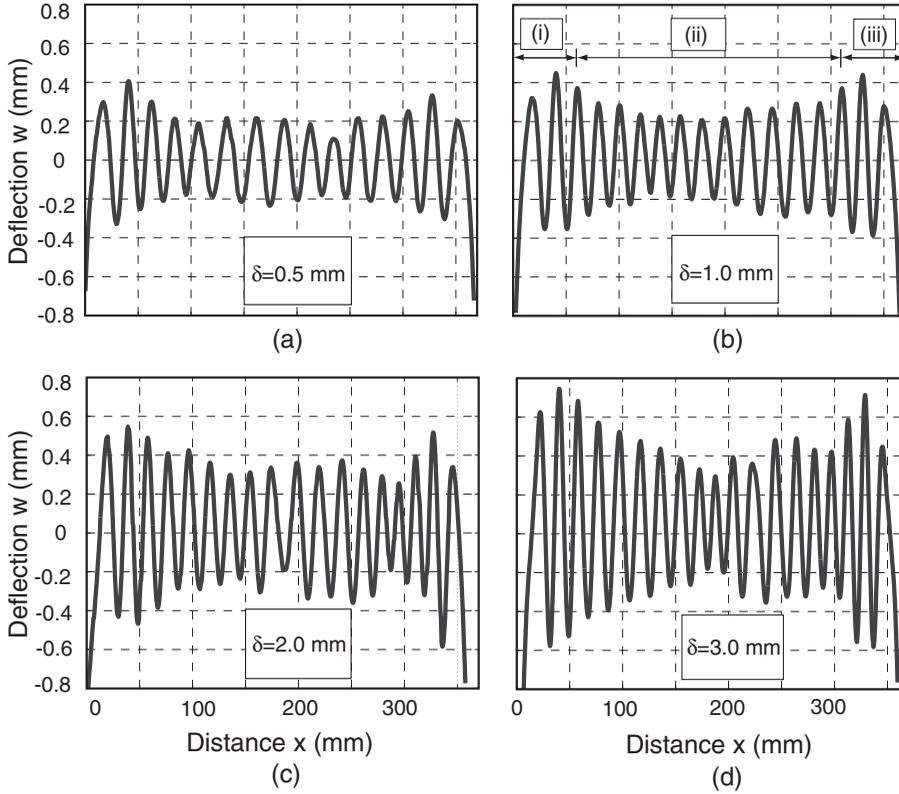
**Figure 4.** Section A-A of 0.025 mm thick Kapton<sup>®</sup> film for shear displacements of (a)  $\delta = 0.5$  mm, (b)  $\delta = 1.0$  mm, (c)  $\delta = 2.0$  mm, and (d)  $\delta = 3.0$  mm.
