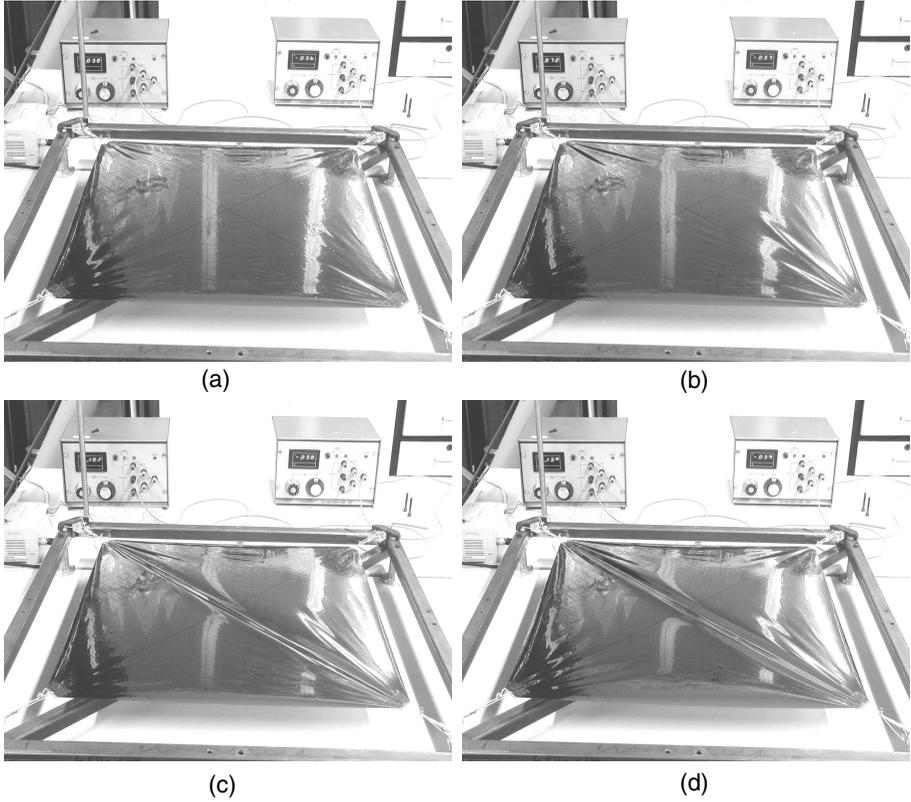
**Figure 10.** Wrinkle pattern in 0.025 mm thick square Kapton<sup>®</sup> membrane for (a)  $T_1/T_2 = 1$ , (b)  $T_1/T_2 = 2$ , (c)  $T_1/T_2 = 3$  and (d)  $T_1/T_2 = 4$ .
