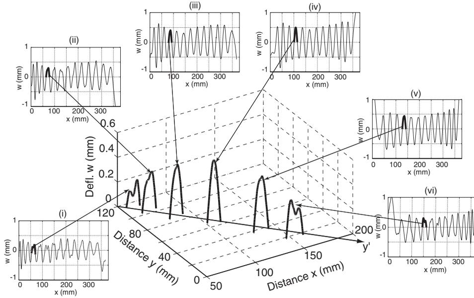
**Figure 6.** Three-dimensional view of half-wrinkle in sheared membrane.
