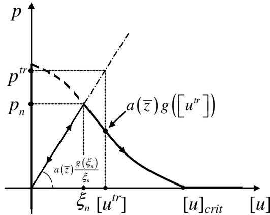
**Figure 4.** Unlimited elastic cohesive law used for computing the trial solution.
