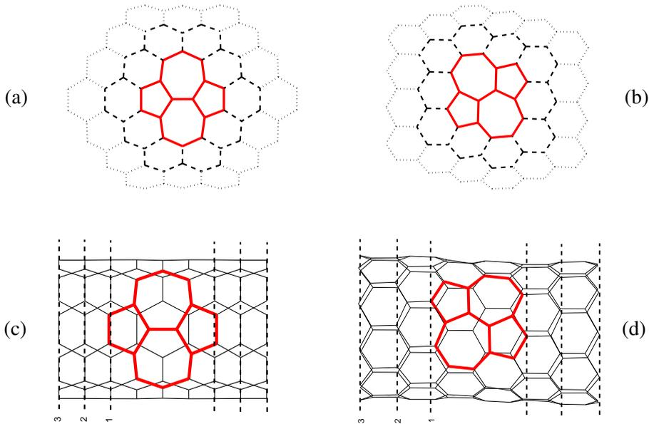
**Figure 1.** Illustration of the defective patches: (a) and (b) are layer models for large diameter tubes; (c) and (d) are ring models for small diameter tubes.
