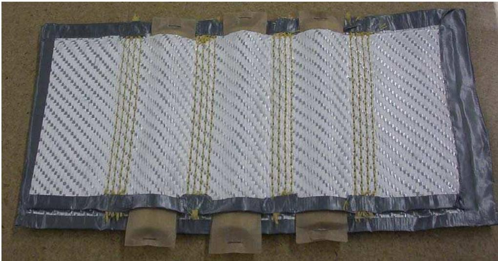
**Figure 7.** Dyneema specimen ready for resin infiltration.
