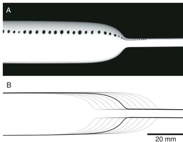
**Figure 5.** (A) Snapshot of the inflated balloon with its fiducial points. (B) Propagation of the growth front during inflation. The velocity of the material entering the front is  $V = 2.55$  mm/s assuming that the front is fixed in space. The velocity of the material that exits the front is  $v_c = \lambda_s^{\max} V = 3.74 \times 2.55$  mm/s = 9.54 mm/sec, where  $\lambda_s^{\max}$  is the maximal meridional stretch.
