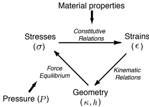
**Figure 8.** Three fundamental relations for thin pressurized shells.
