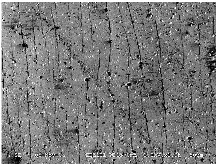
**Figure 1.** WC-DLC coating pulled to 4% strain resulting in longitudinal cracks. Tensile direction is perpendicular (horizontal in the figure) to the longitudinal cracks.
