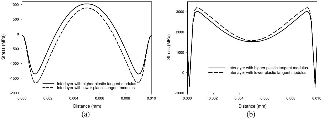
**Figure 11.** Comparison of  $\sigma_{xx}$  stresses between two cracks 10  $\mu\text{m}$  apart for two interlayer cases: (a) stresses at the surface of the coating, and (b) stresses near the coating-interlayer interface.
