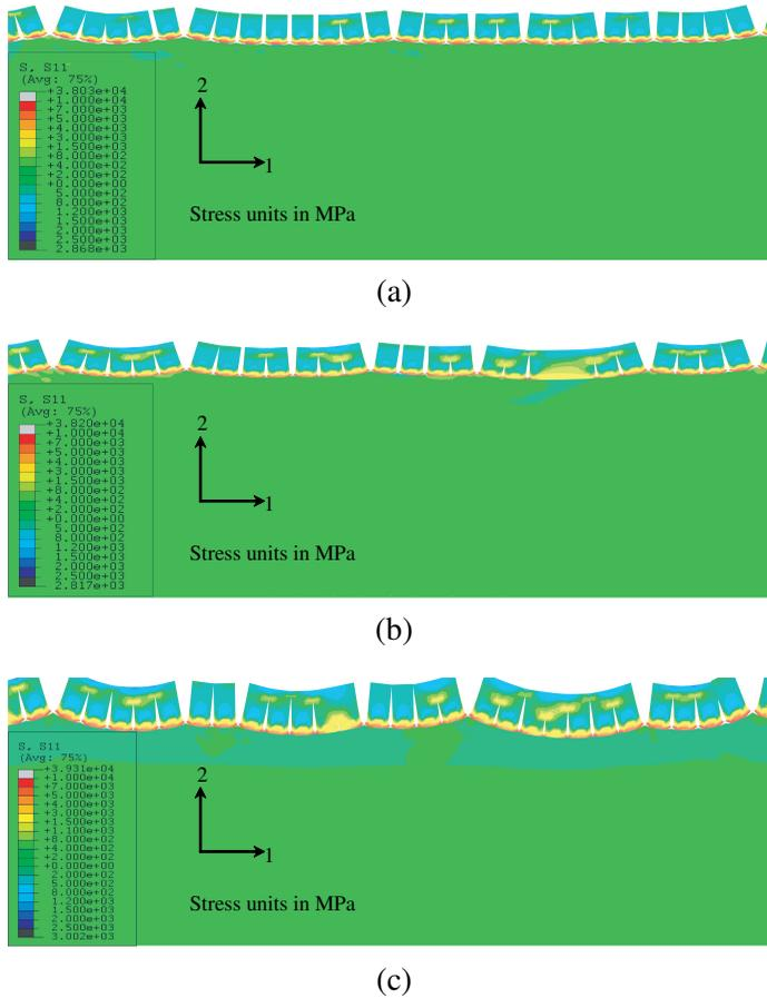
**Figure 10.** Change in cracks from reference model due to: (a) increase in coating modulus; (b) increase in tangent modulus slope in interlayer; and (c) decrease in tangent modulus slope in interlayer. All images correspond to 2.5% strain.
