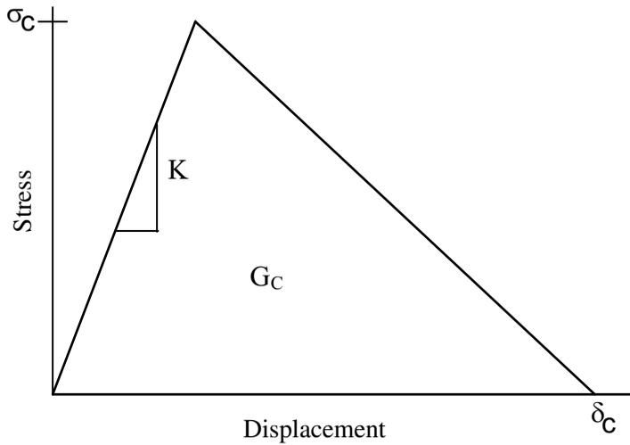
**Figure 4.** Bilinear law followed by the cohesive elements used in the study. Cohesive elements have a stiffness  $K$  and fail when the critical stresses in the elements reach beyond the critical stress  $\sigma_C$ .
