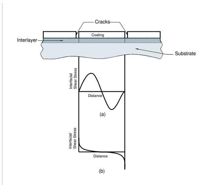
**Figure 2.** Two different theories predicting the distribution of interfacial shear stresses along the coating-interlayer interface between two cracks when the coating-interlayer-substrate system is subject to tensile loads: (a) sinusoidal distribution with zero stress at the endpoints [Agrawal and Raj 1989], and (b) maximum stress at the endpoints [Chen et al. 2000; Yanaka et al. 1998; Wojciechowski and Mendolia 1989].
