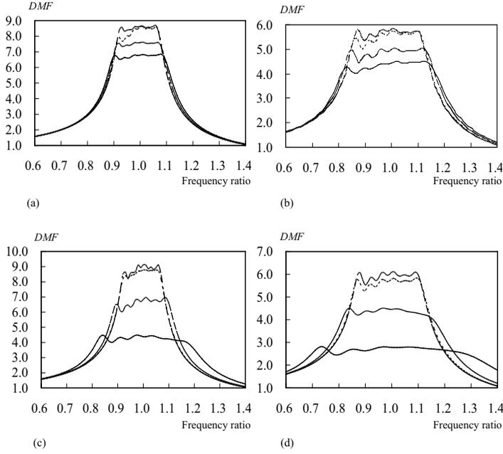
**Figure 8.** FRFs of the structures with the LT-AMTMD with  $n = 5$ ,  $\alpha = 0.4$ ,  $\mu = 0.01$ , and several  $\beta$  values (considering the changes of actuator locations) and with (a)  $r = -0.4$  and  $\mu_T = 0.01$ ; (b)  $r = -0.4$  and  $\mu_T = 0.03$ ; (c)  $r = -0.8$  and  $\mu_T = 0.01$ ; and (d)  $r = -0.8$  and  $\mu_T = 0.03$ . Legend: —  $\beta = 0.0$ ; - -  $\beta = 0.36$ ; ···  $\beta = 0.86$ ; - · -  $\beta = 1.0$ .
