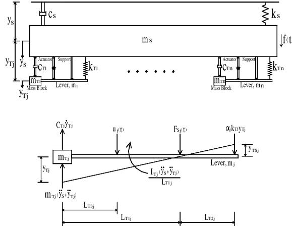
**Figure 1.** Schematic diagram of the lever-type active multiple tuned mass dampers (LT-AMTMD) structure system under the external excitation directly acting on the structure rather than through the base.
