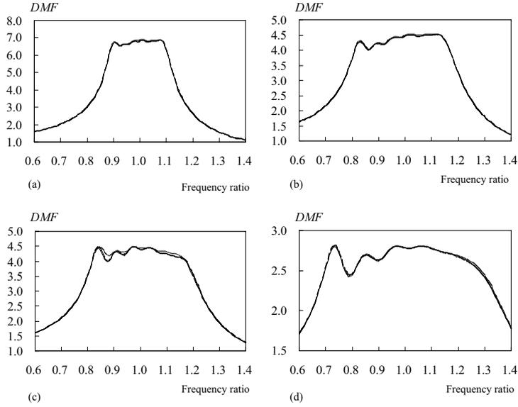
**Figure 6.** FRFs of the structures with the LT-AMTMD with the actuator set at the mass block with  $n = 5$ ,  $\mu = 0.01$ , and several  $\alpha$  values (considering the changes of the support locations) and with (a)  $r = -0.4$  and  $\mu_T = 0.01$ ; (b)  $r = -0.4$  and  $\mu_T = 0.03$ ; (c)  $r = -0.8$  and  $\mu_T = 0.01$ ; and (d)  $r = -0.8$  and  $\mu_T = 0.03$ . Legend:—  $\alpha = 0.1$ ; --  $\alpha = 0.3$ ; ---  $\alpha = 0.5$ ; -.-  $\alpha = 1.0$
