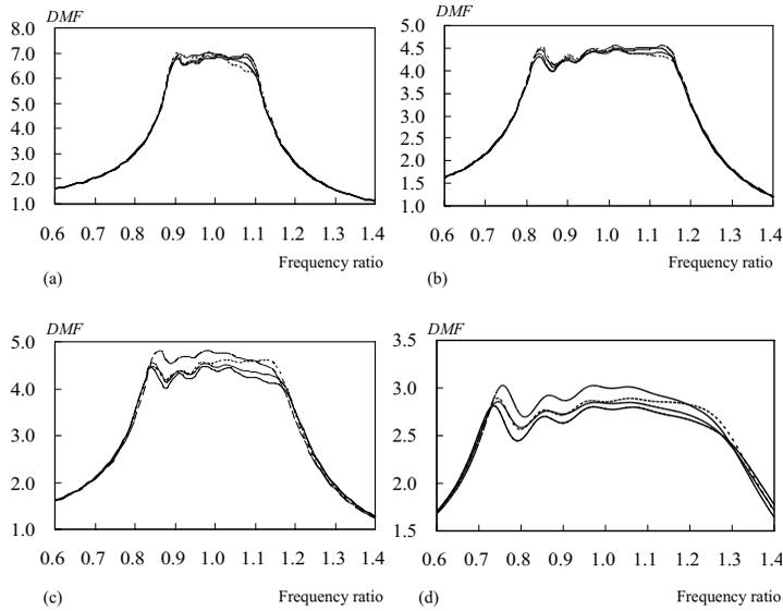
**Figure 7.** FRFs of the structures with the LT-AMTMD with the actuator set at the mass block with  $n = 5$ ,  $\alpha = 0.4$ , and several  $\mu$  values (considering the changes of lever mass) and with (a)  $r = -0.4$  and  $\mu_T = 0.01$ ; (b)  $r = -0.4$  and  $\mu_T = 0.03$ ; (c)  $r = -0.8$  and  $\mu_T = 0.01$ ; and (d)  $r = -0.8$  and  $\mu_T = 0.03$ . Legend:—  $\mu = 0.01$ ; --  $\mu = 0.05$ ; ---  $\mu = 0.10$ ; -.-  $\mu = 0.20$ .
