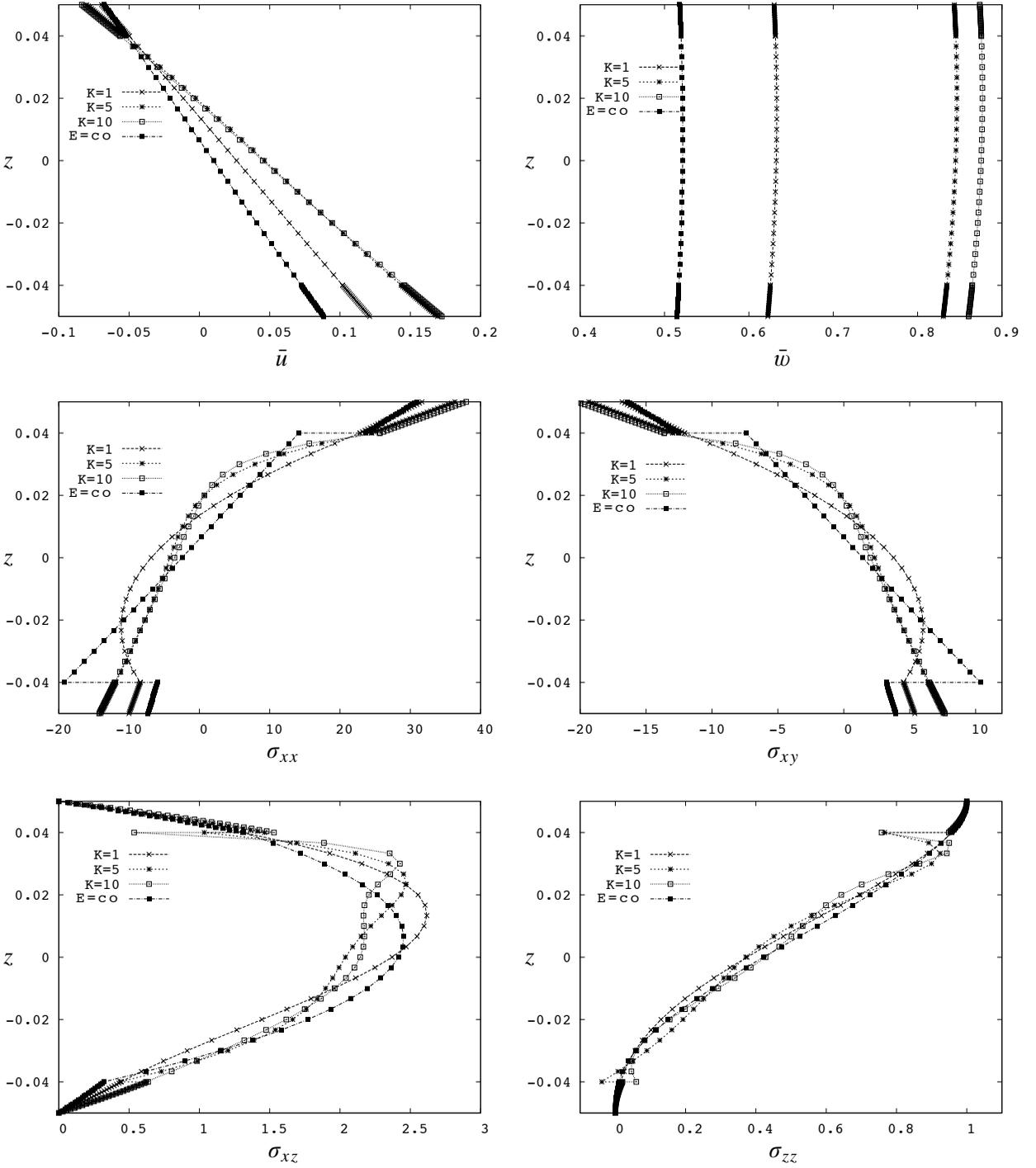
**Figure 10.** Benchmark: For the sandwich plate with core in FGM, displacements  $(\bar{u}, \bar{w}) = 10(u_x, u_z)E_c h^3 / (\bar{p}_z a^4)$  and stresses  $\sigma_{xx}$ ,  $\sigma_{xy}$ ,  $\sigma_{xz}$  and  $\sigma_{zz}$  versus  $z$  for LD4 theory. In addition to the values  $\kappa = 1, 5, 10$  in Zenkour’s formula (19), we consider an isotropic material with  $E = 225$  GPa for the core (“E = co”). Thickness ratio:  $a/h = 10$ .
