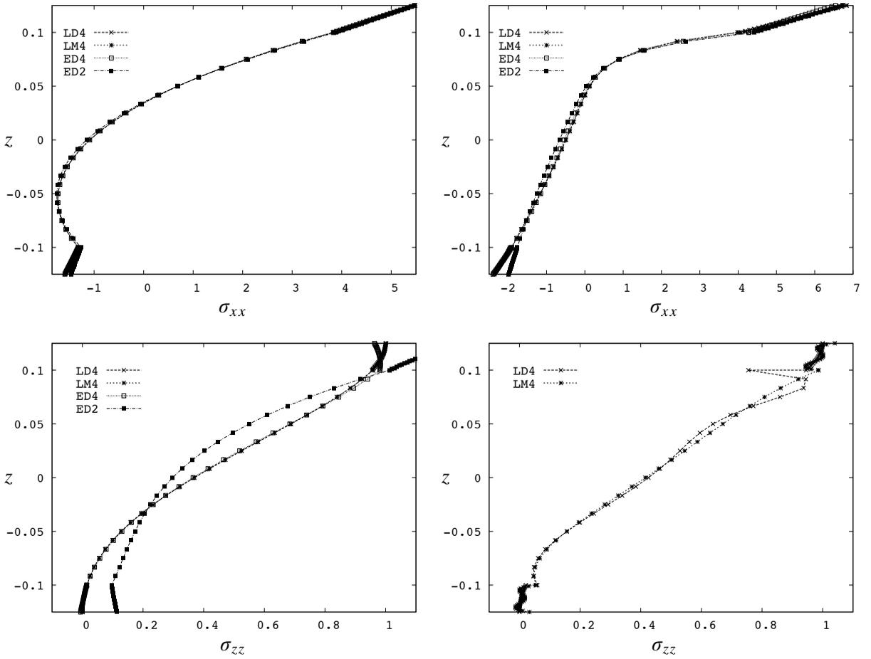
**Figure 9.** Benchmark: Sandwich plate with core in FGM. In-plane stress  $\sigma_{xx}$  (top row) and transverse-normal stress  $\sigma_{zz}$  (bottom row) versus  $z$  for  $\kappa = 1$  (left) and  $\kappa = 10$  (right). The thickness ratio is  $a/h = 4$ .
