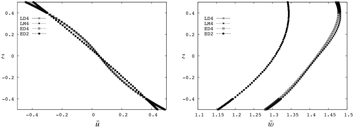
**Figure 6.** Assessment 3: Displacements  $\bar{u} = G_0 u_x / (\bar{p}_z h_0)$  and  $\bar{w} = G_0 u_z / (\bar{p}_z h_0)$  vs.  $z$ , for the sandwich plate with core in FGM proposed in [Kashtalyan and Menshykova 2009]. The shear modulus is  $G_c/G_f = 0.9$ .
