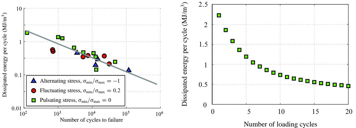
**Figure 10.** Left: experimental results for dissipated energy per cycle as a function of the number of cycles to failure, for  $\alpha = 11$  and  $\beta = -0.377$ , and fit using Equation (15). Right: numerical results for dissipated energy per cycle with respect to the number of cycles, with  $\Delta\sigma = 400\text{Mpa}$ .
