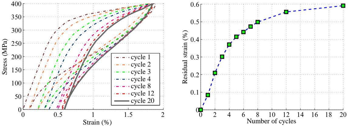
**Figure 3.** Left: experimental stress-strain response of a NiTi wire to repeated tension. The stabilized cycle is shown by a continuous line. Right: residual strain evolution with respect to the number of tension cycles.
