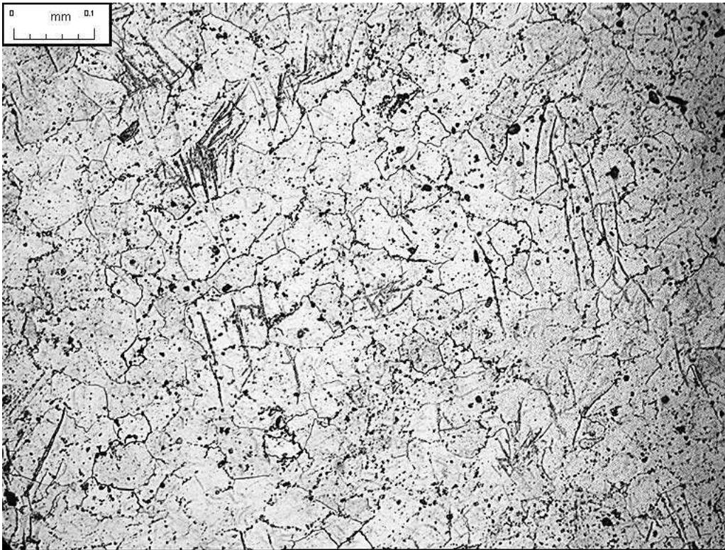
**Figure 6.** Metallographic structure of the NiTi alloy.
