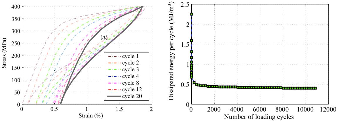
**Figure 9.** Left: experimental stabilization of the amount of dissipated energy per cycle,  $W_d$ , with the number of cycles. Right: dissipated energy per cycle versus number of loading cycles: experimental result for  $\Delta\sigma = 400\text{Mpa}$ .
