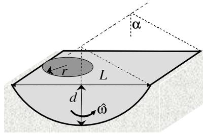
**Figure 6.** Plane strain circular rigid body virtual collapse mechanism.
