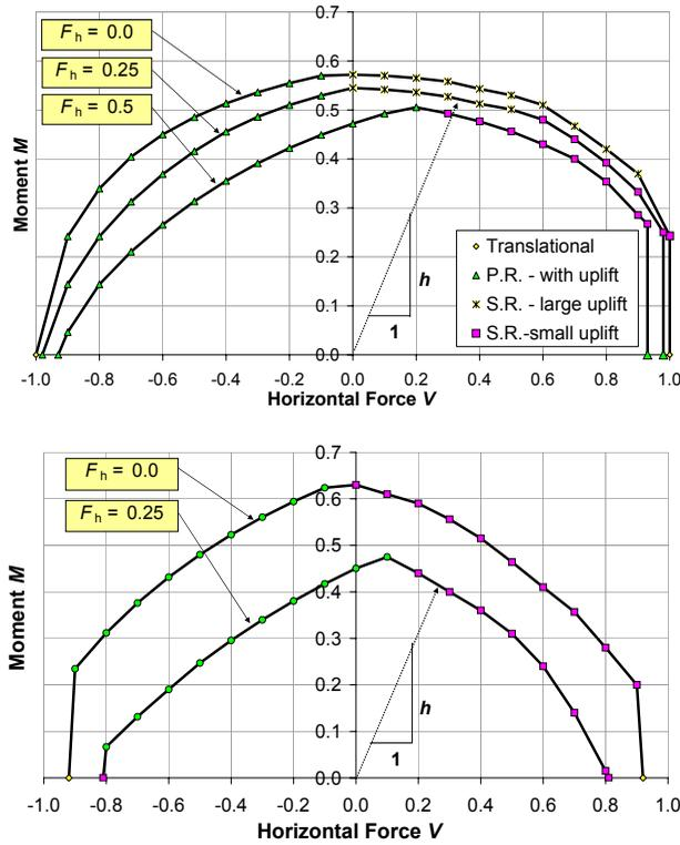
**Figure 9.** Tresca criterion with zero tension cut-off: interaction diagram ( $\tilde{N} = \text{const}$ ,  $\tilde{V}$ ,  $\tilde{M}$ ,  $\tilde{F}_h$ ) for  $\tilde{k} = 0$ ,  $\tilde{N}_{\max}^0/\tilde{N} > 3$  (top) and  $\tilde{N}_{\max}^0/\tilde{N} > 1.5$  (bottom); ultimate loading paths for  $\tilde{F}_h = 0.25$  in a SDOF superstructure.
