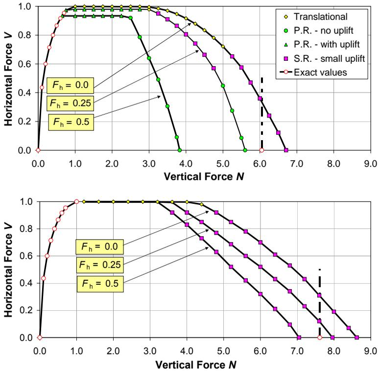
**Figure 8.** Interaction diagram ( $\tilde{N}$ ,  $\tilde{V}$ ,  $\tilde{M} = 0$ ,  $\tilde{F}_h$ ) for  $\tilde{k} = 0$  (top) and  $\tilde{k} = 1$  (bottom). Tresca criterion with zero tension cut-off.
