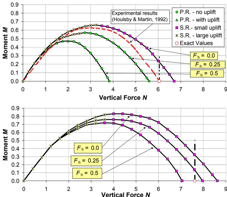
**Figure 10.** Interaction diagram ( $\tilde{N}$ ,  $\tilde{V} = 0$ ,  $\tilde{M}$ ,  $\tilde{F}_h$ ) for  $\tilde{k} = 0$  (top) and  $\tilde{k} = 1$  (bottom), and experimental results by Houlsby and Martin [1993]. Tresca criterion with zero tension cut-off.
