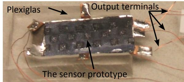
**Figure 11.** Photograph of the microfabricated prototype sensor.
