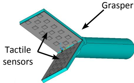
**Figure 4.** The proposed sensor after assembly and integration with an endoscopic MIS tool. A single sensor may be integrated with one jaw, or each jaw may be provided with its own sensor, allowing the combined signal to offer additional tactile information such as the depth of embedded lumps.
