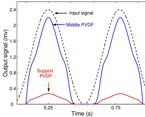
**Figure 17.** Experimental values of generated voltage on the support and middle sensing elements when a sinusoidal point load of amplitude 10 mN and frequency 2 Hz was applied on the middle of the sensor.
