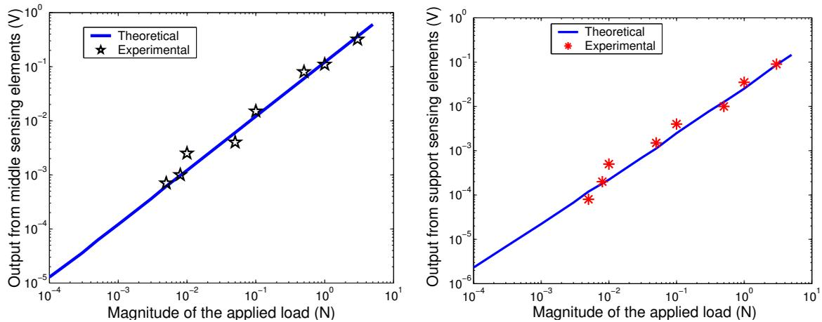
**Figure 13.** Left: calibration curve of the middle PVDF-sensing element. Right: calibration curve of each sensing element at the supports. For both curves, the experimental applied point loads ranged from 1 mN to 3 N and were always applied at the center of the sensor.
