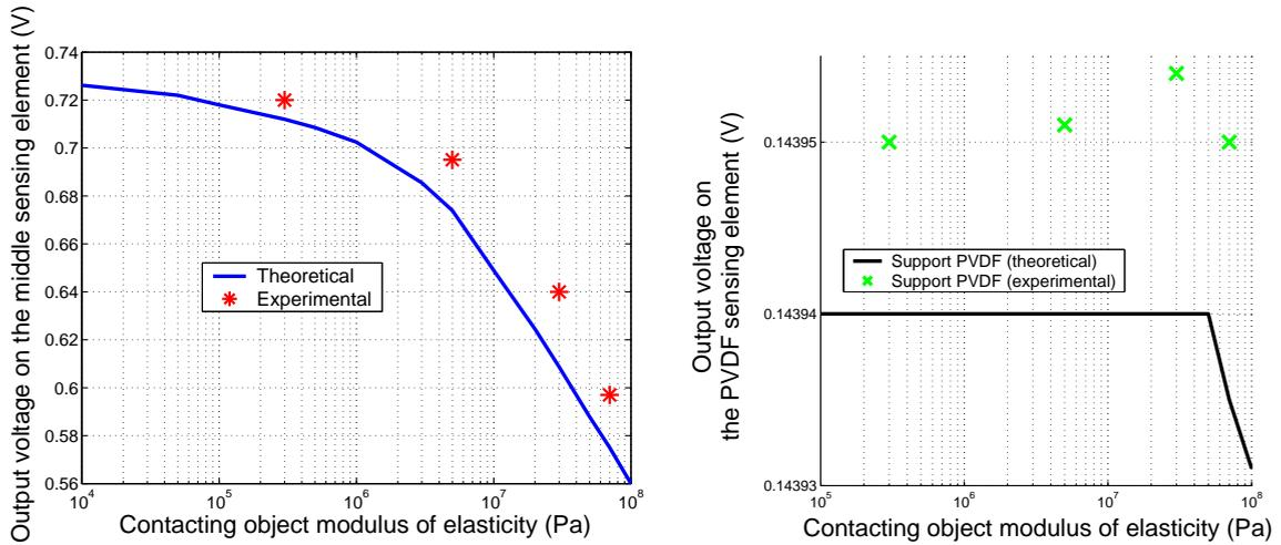
**Figure 16.** Theoretical and experimental values of the generated voltage on the sensing elements versus different modulus of elasticity of the contacting tissue, under application of a 5 N distributed uniform load. Left: middle sensing element. Right: support sensing element.
