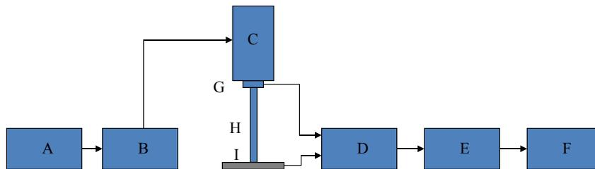
**Figure 12.** Experimental setup diagram: (A) signal generator, (B) power amplifier, (C) vibrator, (D) charge and voltage amplifiers, (E) A/D converter, (F) computer, (G) force transducer, (H) probe, and (I) the proposed sensor under test.
