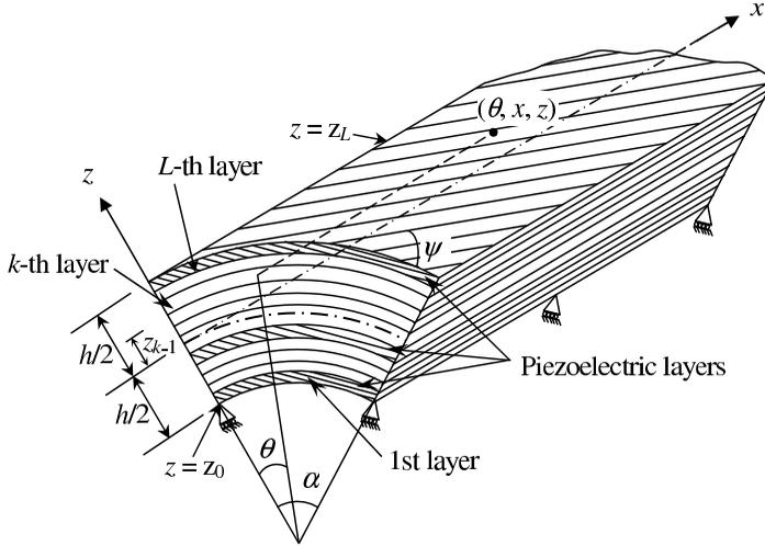
**Figure 1.** Geometry of a hybrid angle-ply cylindrical shell.
