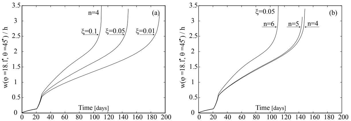
**Figure 10.** Varying stiffness imperfection (scenario 3): (a) variation in time of peak deflection with  $n = 4$  and different imperfection amplitudes; (b) variation in time of peak deflection with  $\xi = 0.05$  and different circumferential wave numbers.
