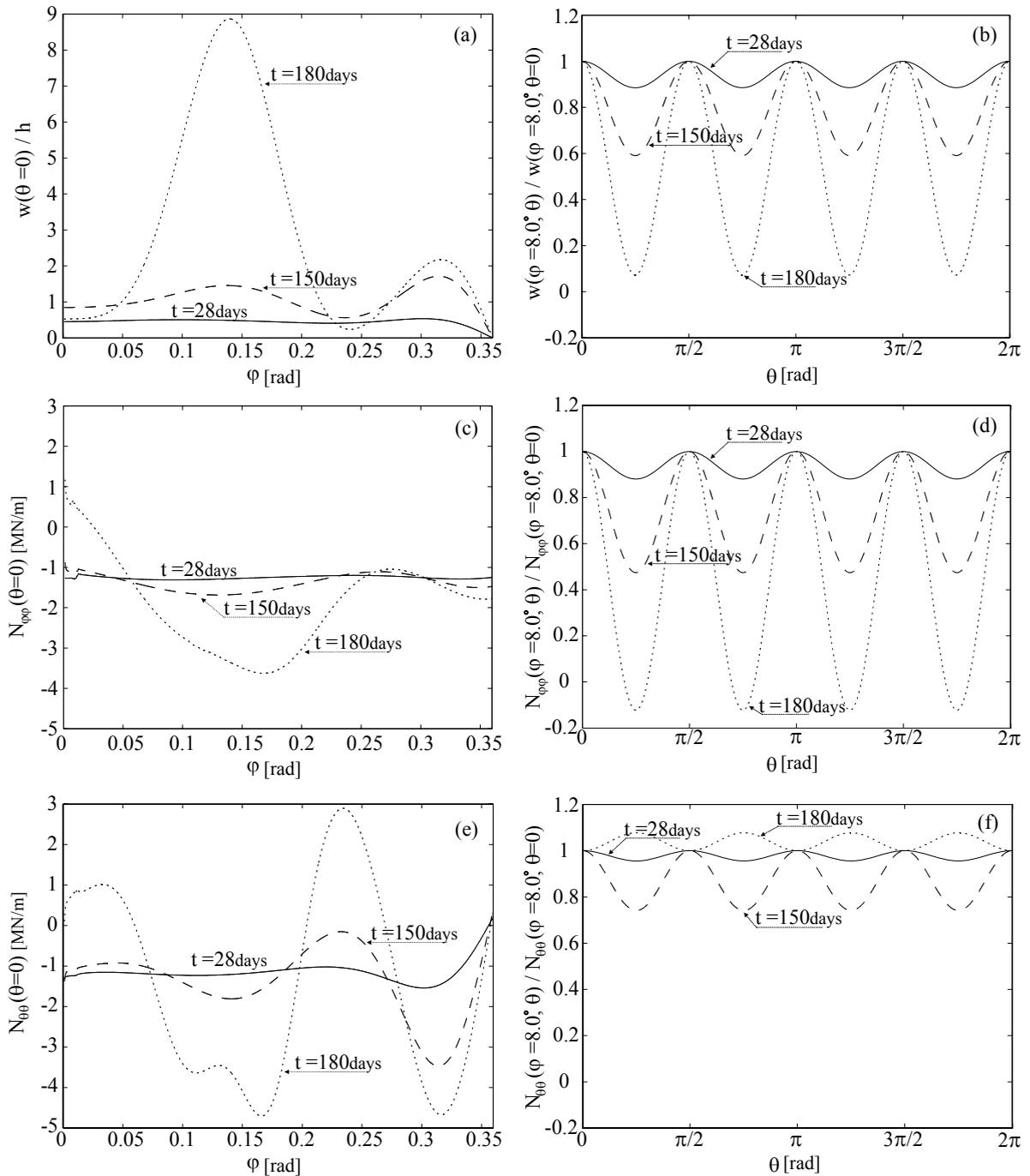
**Figure 8.** Structural response at three different times of a dome with nonaxisymmetric geometric imperfection ( $\zeta = 0.05$ ,  $n = 4$ ): (a, b) perpendicular deformation; (c, d) radial force; (e, f) circumferential force. Solid line:  $t = 28$  days; dashed line:  $t = 150$  days; dotted line:  $t = 180$  days.
