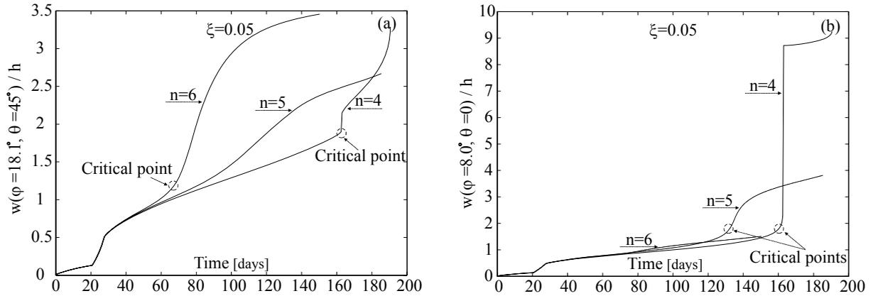
**Figure 9.** Behaviour in time under nonaxisymmetric imperfection (scenario 2) with  $\xi = 0.05$  and different circumferential wave numbers: (a) deflection at  $\varphi = 18.1^\circ$  and  $\theta = 45^\circ$ ; (b) deflection at  $\varphi = 8.0^\circ$  and  $\theta = 0^\circ$ .
