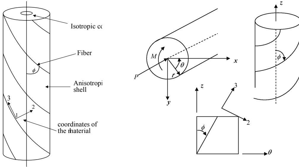
**Figure 3.** Helicoidal structure and its coordinate system.
