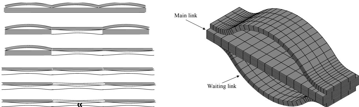
**Figure 1.** Left: A chain of bistable structures and their damage process. Gray regions represent the undamaged main strips. The broken main strips are shown in white. Right: A bistable structure with a symmetric waiting element.
