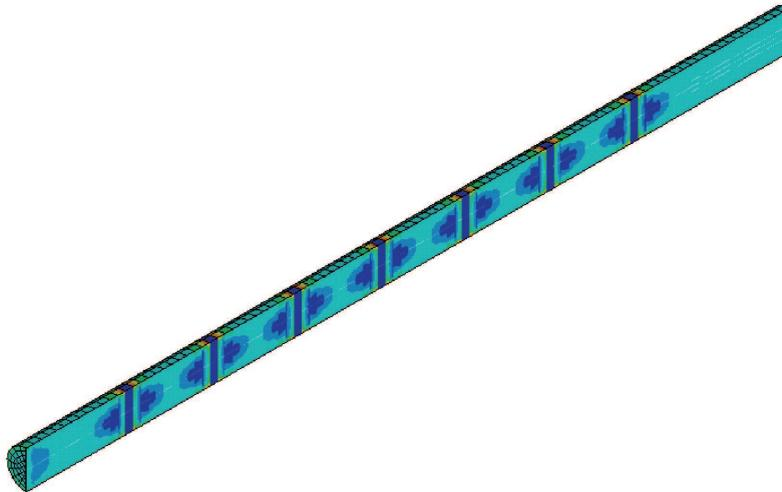
**Figure 8.** Contour plot of normalized von Mises stress in the main link when the breakage locations are 50.8 mm apart. Darker (blue) areas correspond to values near 0 and lighter areas to values near 0.3.
