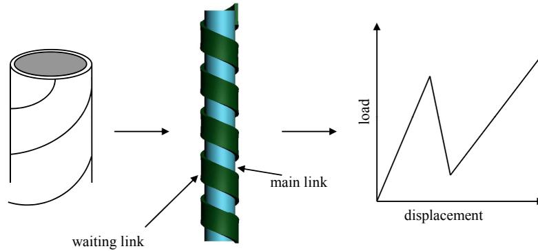
**Figure 2.** Representative model of a helicoidal bistable structure.
