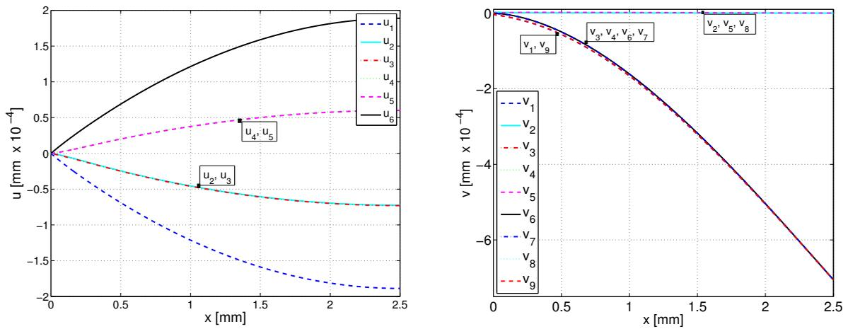
**Figure 4.** Axial displacements  $\hat{u}$  (left) and transverse displacements  $\hat{v}$  (right) as functions of  $x$  for a three-layer homogeneous cantilever, clamped at  $x = 0$ , loaded at  $x = 2.5$  by a quadratic shear distribution, and modeled with 64 elements.
