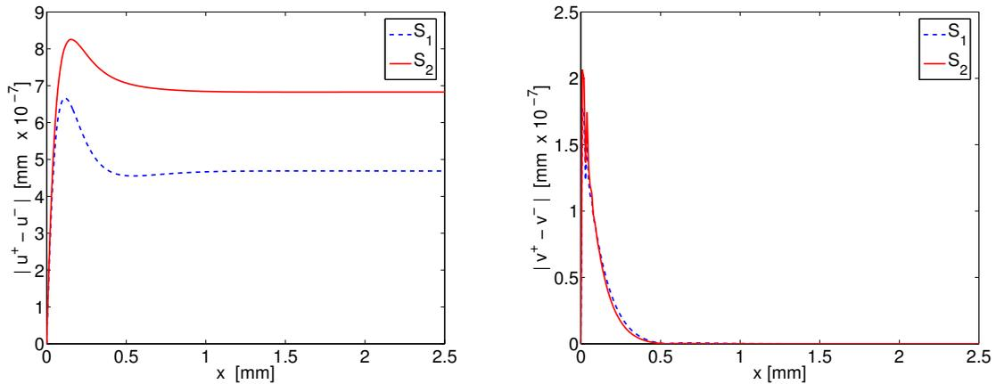
**Figure 7.** Compatibility mismatches on interlayer surfaces  $y = -\frac{1}{5}$  (labeled  $S_1$ ) and  $y = \frac{1}{6}$  ( $S_2$ ): axial displacement jump  $|u(x)^+ - u(x)^-|$  (left) and transverse displacement jump  $|v(x)^+ - v(x)^-|$  (right).
