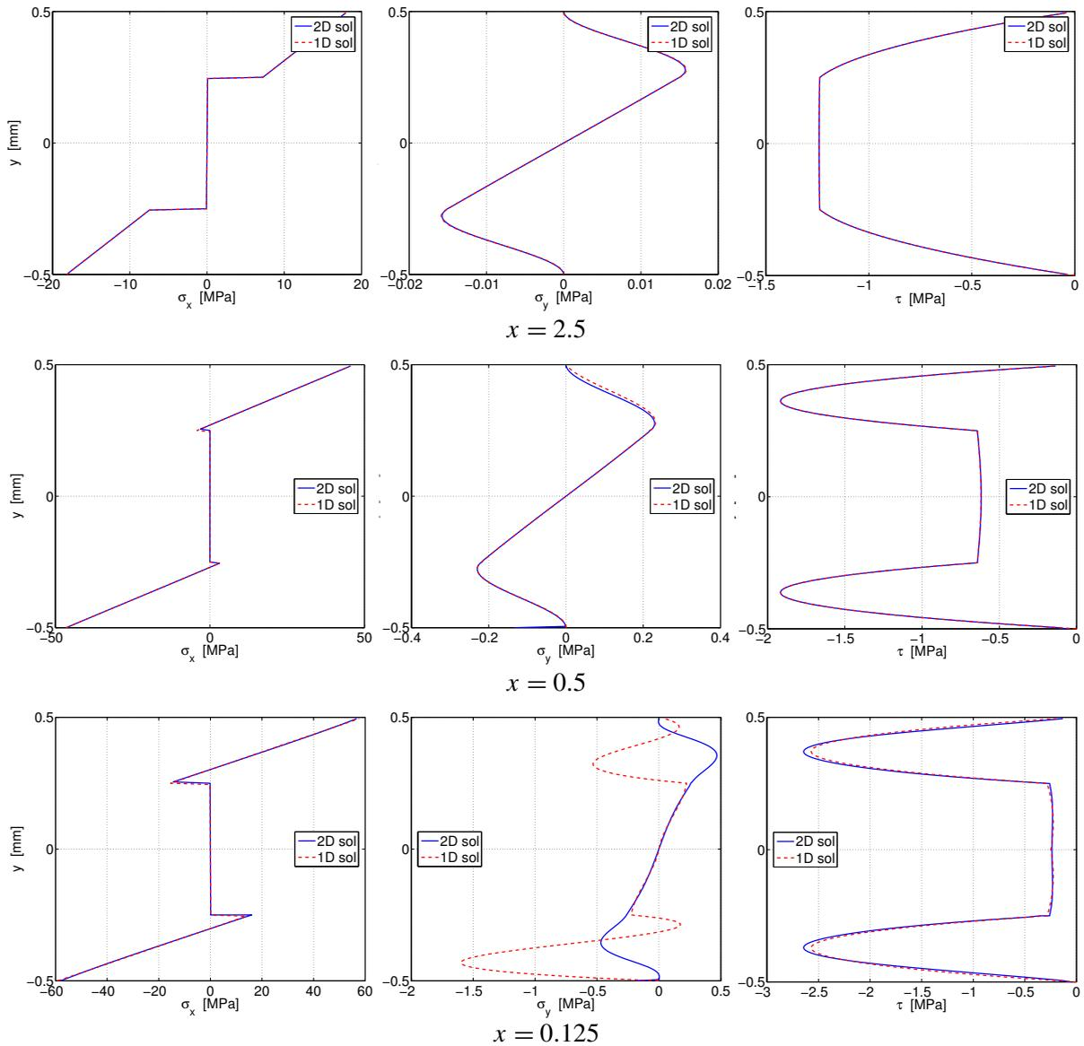
**Figure 8.** Cross-section stresses  $\sigma_x$  (left),  $\sigma_y$  (middle), and  $\tau$  (right), as functions of  $y$ : one- and two-dimensional solutions for the symmetric section. Three cross-sections are considered, at various distances from the clamped boundary: far ( $x = -2.5$ , top), close ( $x = 0.5$ , middle), and very close ( $x = 0.125$ , bottom).
