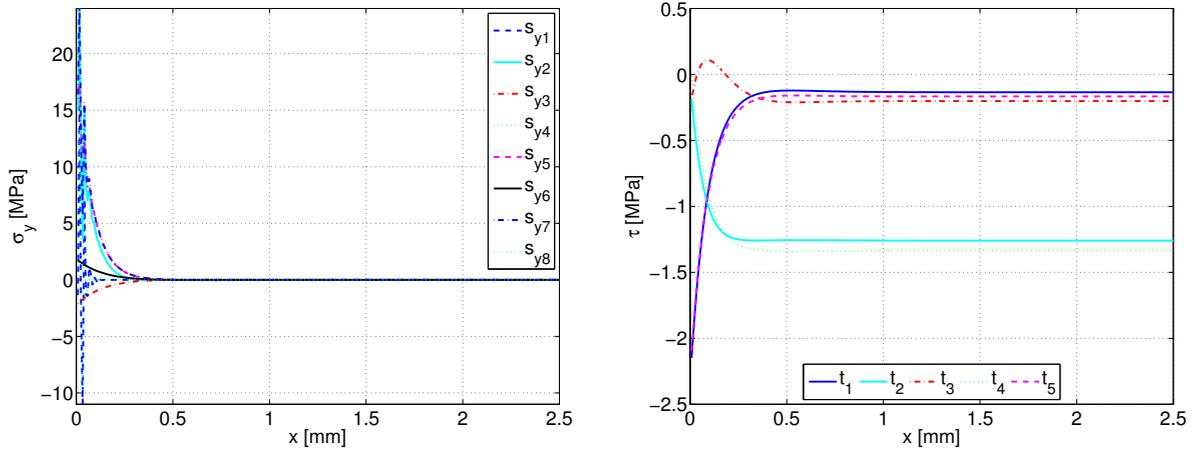
**Figure 6.** Transverse compressive stress  $\hat{\sigma}_y$  (left) and shear stress  $\hat{\tau}$  (right) as functions of  $x$  for a three-layer homogeneous cantilever, clamped at  $x = 0$ , loaded at  $x = 2.5$  by a quadratic shear distribution, and modeled with 64 elements.
