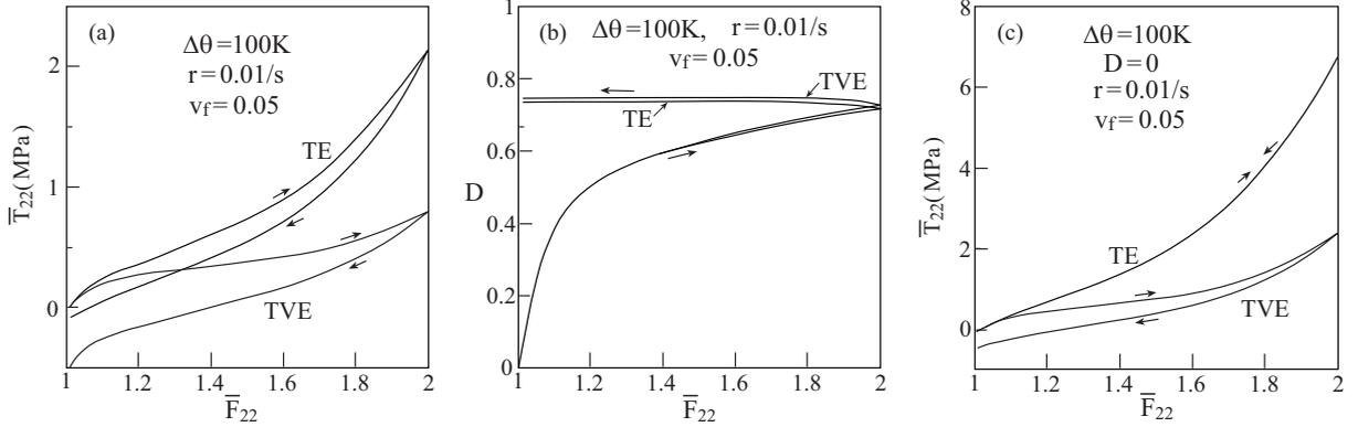
**Figure 5.** Response of the steel/rubber-like thermoviscoelastic (TVE) and thermoelastic (TE) composite to uniaxial stress loading in the transverse 2-direction, applied at elevated temperature  $\Delta\theta = 100$  K at a rate of  $r = \dot{\bar{F}}_{22} = 0.01/s$ : global stress-deformation gradient response (a), damage evolution (b), and global stress-deformation gradient response in the absence of damage (c).
