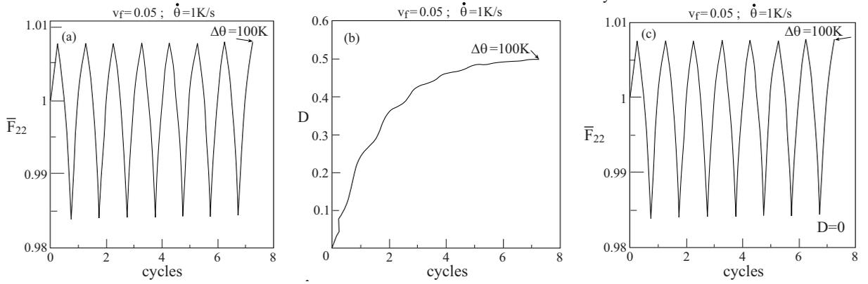
**Figure 7.** Response of the thermoviscoelastic steel/rubber-like composite that is subjected to cyclic thermal loading  $-100 \text{ K} \leq \Delta\theta \leq 100 \text{ K}$  at a rate of  $\dot{\theta} = 1 \text{ K/s}$ , while keeping it traction-free: transverse deformation gradient variation with cycles (a), damage evolution with cycles (b), and transverse deformation gradient variation with cycles in the absence of damage (c).
