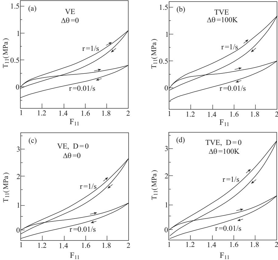
**Figure 4.** Top row: stress-deformation gradient response of the homogeneous viscoelastic (a) and thermoviscoelastic (b) rubber-like material to uniaxial stress loading in the 1-direction, applied at two rates:  $r = \dot{F}_{11} = 1/s$  and  $0.01/s$ . In (a) the VE material is kept at  $\theta = \theta_0$ , in (b) the TVE material undergoes a temperature change of  $\Delta\theta = 100$  K. Bottom row: corresponding results in the absence of damage effects.
