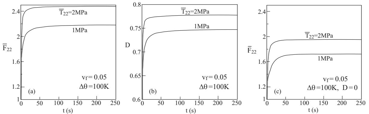
**Figure 10.** Comparison between the creep behaviors of the thermoviscoelastic steel/rubber-like composite which is subjected to uniaxial transverse stress loadings  $\bar{T}_{22} = 1 \text{ MPa}$  and  $2 \text{ MPa}$  at elevated temperature  $\Delta\theta = 100 \text{ K}$ . As functions of time, the plots show the global transverse deformation gradient (a), damage evolution (b), and global transverse deformation gradient in the absence of damage effects.
