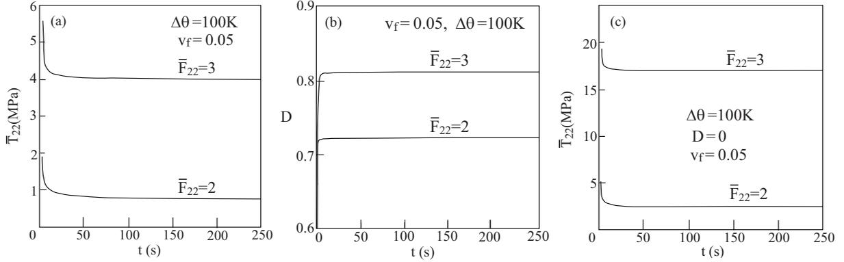
**Figure 14.** Comparison between the relaxation behaviors of the thermoviscoelastic steel/rubber-like composite which is subjected to uniaxial transverse stress loadings such that  $\bar{F}_{22} = 2$  and 3 at elevated temperature  $\Delta\theta = 100$  K. Global transverse stress (a), damage evolution (b), and global transverse stress in the absence of damage effects (c).
