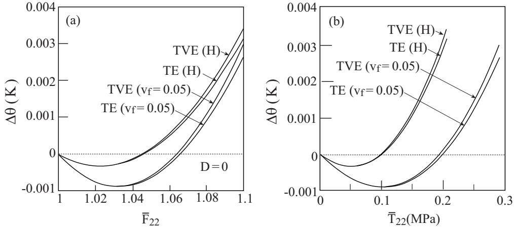
**Figure 2.** Temperature deviations generated by applying, under isentropic conditions, a uniaxial transverse stress loading on thermoviscoelastic (TVE) and thermoelastic (TE) composites. Also shown are the corresponding temperature deviations generated in the homogeneous (H) unreinforced matrix. The minima correspond to the locations of the thermoelastic inversions. Temperature deviations are plotted against average transverse deformation gradient (a) and against average transverse stress (b).
