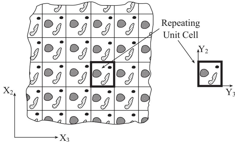
**Figure 1.** A multiphase composite with doubly periodic microstructures defined with respect to global initial coordinates of the plane  $X_2 - X_3$ . The repeating unit cell is defined with respect to local initial coordinates of the plane  $Y_2 - Y_3$ .
