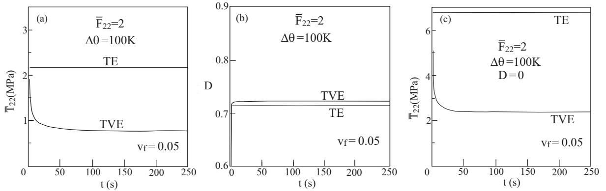
**Figure 15.** Comparison between the relaxation behaviors of thermoviscoelastic (TVE) and thermoelastic (TE) steel/rubber-like composites where in the latter the viscous effects of in the matrix phase have been neglected. Both composites are subjected to uniaxial transverse stress loading such that  $\bar{F}_{22} = 2$  at elevated temperature  $\Delta\theta = 100$  K. Global transverse stress (a), damage evolution (b), and global transverse stress in the absence of damage effects (c).
