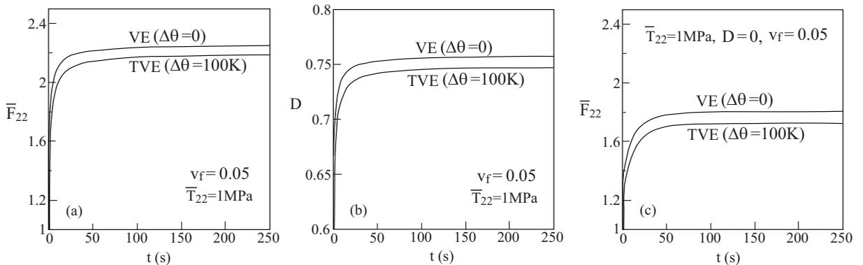
**Figure 12.** Comparison between the creep behaviors of thermoviscoelastic (TVE) at elevated temperature  $\Delta\theta = 100 \text{ K}$ , and viscoelastic (VE) at the reference temperature ( $\Delta\theta = 0$ ) of steel/rubber-like composites. Both are subjected to uniaxial transverse stress loading  $\bar{T}_{22} = 1 \text{ MPa}$ . Global transverse deformation gradient (a), damage evolution (b), and global transverse deformation gradient in the absence of damage effects (c).
