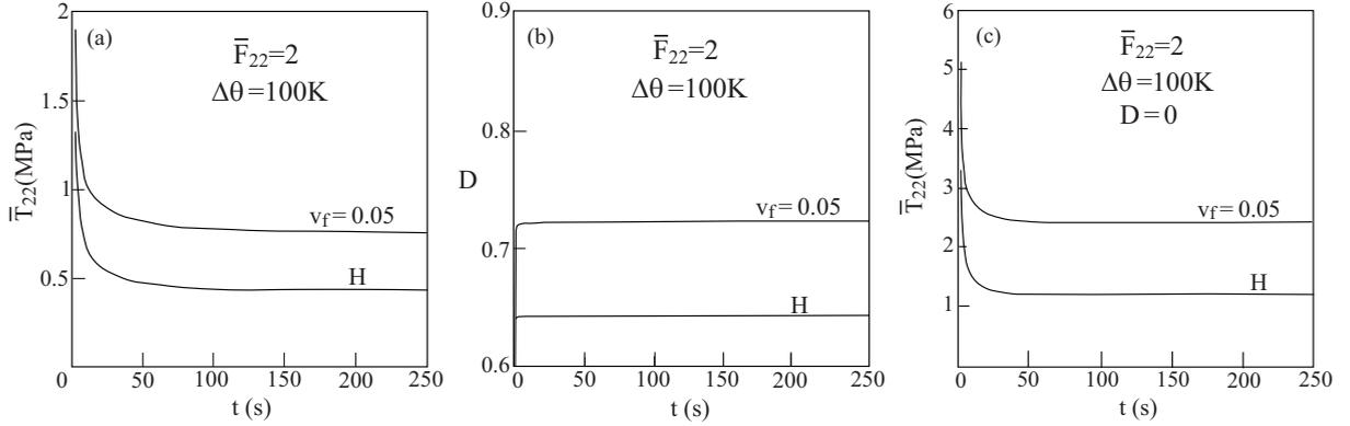
**Figure 13.** Relaxation behavior of the thermoviscoelastic steel/rubber-like composite which is subjected to a uniaxial transverse stress loading such that  $\bar{F}_{22} = 2$  at elevated temperature  $\Delta\theta = 100\text{K}$ . Also shown is the corresponding relaxation behavior of the homogeneous (H) unreinforced thermoviscoelastic matrix. Global transverse stress (a), damage evolution (b), and global transverse stress in the absence of damage effects (c).
