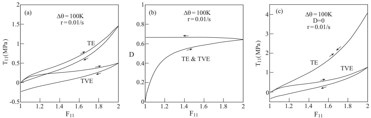
**Figure 3.** Response of the homogeneous thermoviscoelastic (TVE) and thermoelastic (TE) rubber-like material to uniaxial stress loading in the 1-direction, applied at elevated temperature  $\Delta\theta = 100$  K at a rate of  $r = \dot{F}_{11} = 0.01/s$ : stress-deformation gradient response (a), damage evolution (b), and stress-deformation gradient response in the absence of damage (c).
