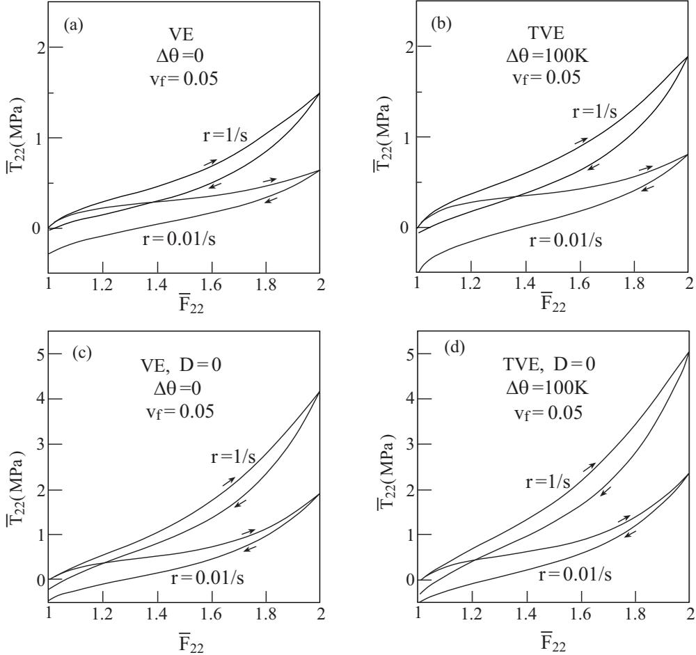
**Figure 6.** Top row: global stress-deformation gradient response of the steel/rubber-like viscoelastic and thermoviscoelastic composite to uniaxial stress loading in the transverse 2-direction, applied at two rates:  $r = \dot{\bar{F}}_{22} = 1/s$  and  $0.01/s$ . In (a) the VE material is kept at  $\theta = \theta_0$ , in (b) the TVE material undergoes a temperature change of  $\Delta\theta = 100$  K. Bottom row: corresponding results in the absence of damage effects.
