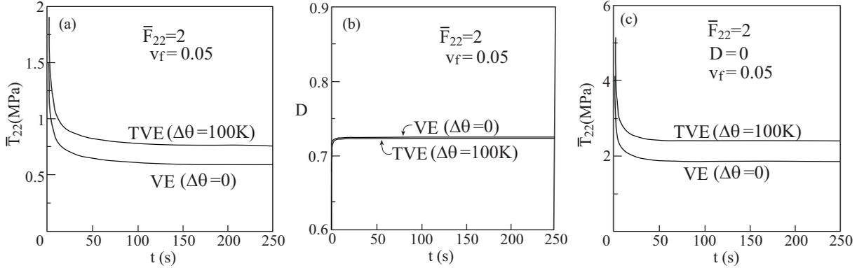
**Figure 16.** Comparison between the relaxation behaviors of thermoviscoelastic (TVE) at elevated temperature  $\Delta\theta = 100$  K, and viscoelastic (VE) at the reference temperature ( $\Delta\theta = 0$ ) of steel/rubber-like composites. Both composites are subjected to uniaxial transverse stress loading such that  $\bar{F}_{22} = 2$ . Global transverse stress (a), damage evolution (b), and global transverse stress in the absence of damage effects (c).
