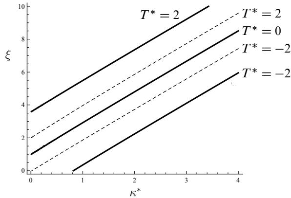
**Figure 5.** Dimensionless squared Rayleigh wave speed  $\xi = \rho v^2/\mu$  versus the parameter  $\kappa^*$  for various values of  $T^*$ , with  $\nu^* = 2.2$ ,  $\gamma^* = 0$ , and  $\lambda^* = 0.15$  (solid lines) or  $\lambda^* = -0.25$  (dashed lines).
