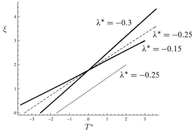
**Figure 4.** Dimensionless squared Rayleigh wave speed  $\xi = \rho v^2/\mu$  versus  $T^*$ , based on (104) and (105), for different values of  $\lambda^*$ . Remaining parameter values are  $\kappa^* = 0.4, \nu^* = 2.2, \gamma^* = 0.5$  (solid lines);  $\kappa^* = 0.4, \nu^* = 2.2, \gamma^* = 0$  (dashed line);  $\kappa^* = 0, \nu^* = 0, \gamma^* = 0$  (dotted line).
