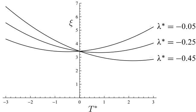
**Figure 3.** Dimensionless squared wave speed  $\xi = \rho v^2/\mu$  versus  $T^*$ , based on (112), for  $\theta = \pi/3, \kappa^* = 0.4, \nu^* = 2.2, \gamma^* = 0.2$  and different values of  $\lambda^*$ .
