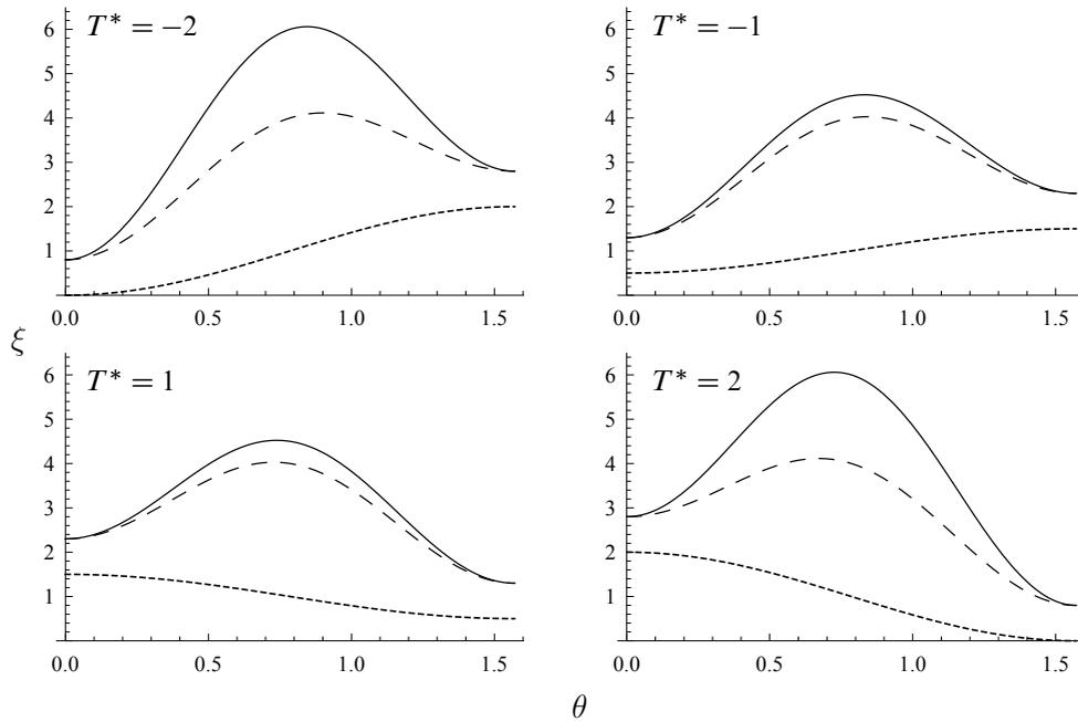
**Figure 2.** Dimensionless squared wave speed  $\xi = \rho v^2/\mu$  versus the angle  $\theta \in [0, \pi/2]$ , based on (112), for  $\lambda^* = -\frac{1}{4}$  and various values of the dimensionless initial stress  $T^*$ . Remaining parameter values are  $\kappa^* = 0.4$ ,  $\nu^* = 2.2$ ,  $\gamma^* = 0.5$  (solid curves);  $\kappa^* = 0.4$ ,  $\nu^* = 2.2$ ,  $\gamma^* = 0$  (thick dashed curves);  $\kappa^* = 0$ ,  $\nu^* = 0$ ,  $\gamma^* = 0$  (thin dashed curves).
