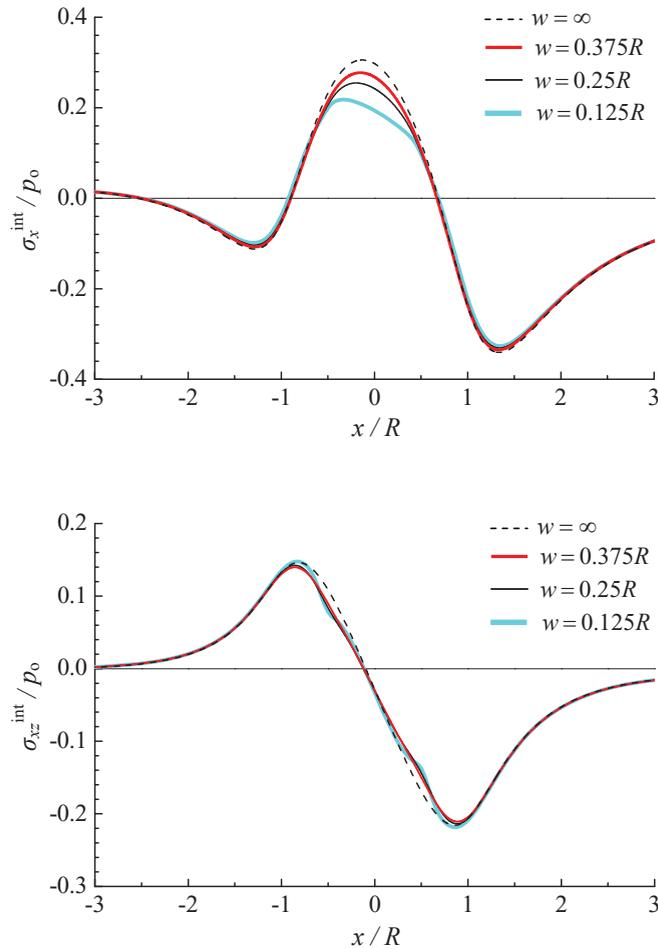
**Figure 5.** Effect of the depths of the inhomogeneity  $\Omega_2$  on the interfacial normal stress  $\sigma_x^{\text{int}}$  (top) and shear stress  $\sigma_{xz}^{\text{int}}$  (bottom) within the coating.
