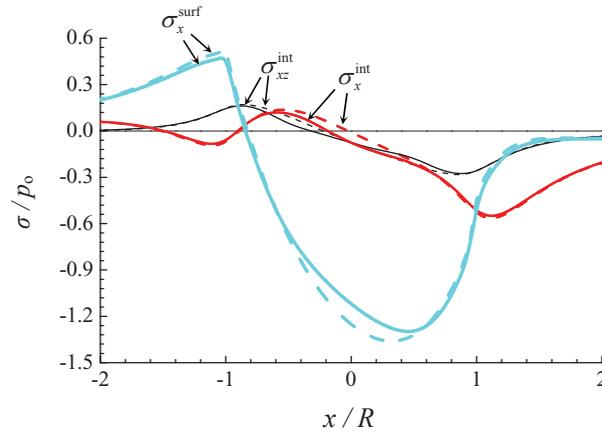
**Figure 7.** The surface stress component  $\sigma_x^{\text{surf}}$  and the interfacial stress components  $\sigma_x^{\text{int}}$  and  $\sigma_{xz}^{\text{int}}$  in the coating of thickness  $H = 0.25R$  along the  $x$ -axis direction.
