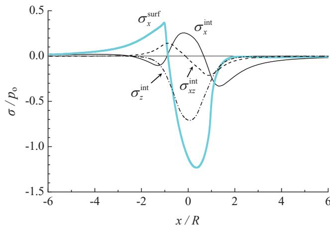
**Figure 3.** The component  $\sigma_x^{\text{surf}}$  of the surface stress and the components  $\sigma_x^{\text{int}}$ ,  $\sigma_z^{\text{int}}$ , and  $\sigma_{xz}^{\text{int}}$  of the interfacial stress in the coating along the  $x$ -axis direction in the computational domain of size  $16R \times 16R \times 1.5R$ .
