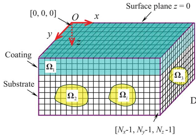
**Figure 1.** Discretization of a computational domain  $D$  into  $N_x \times N_y \times N_z$  cuboids. The domain  $D$  contains  $n$  arbitrarily shaped inhomogeneities in an isotropic half-space, where  $\Omega_1$  is used to model a layer of coating on the substrate matrix.
