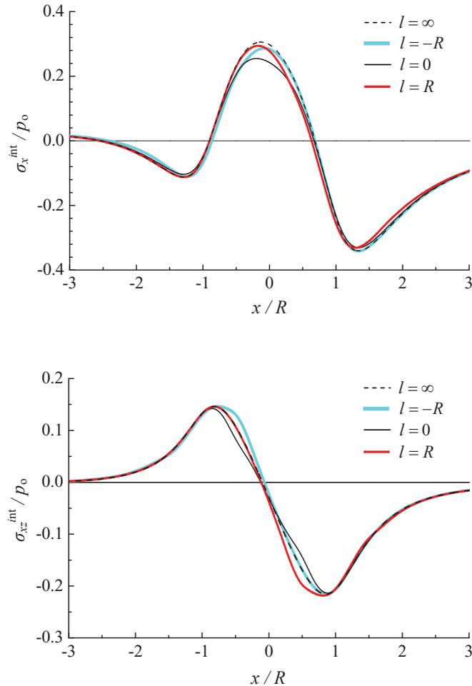
**Figure 4.** Effect of the horizontal position of the inhomogeneity  $\Omega_2$  on the interfacial normal stress  $\sigma_x^{\text{int}}$  (top) and shear stress  $\sigma_{xz}^{\text{int}}$  (bottom) within the coating.
