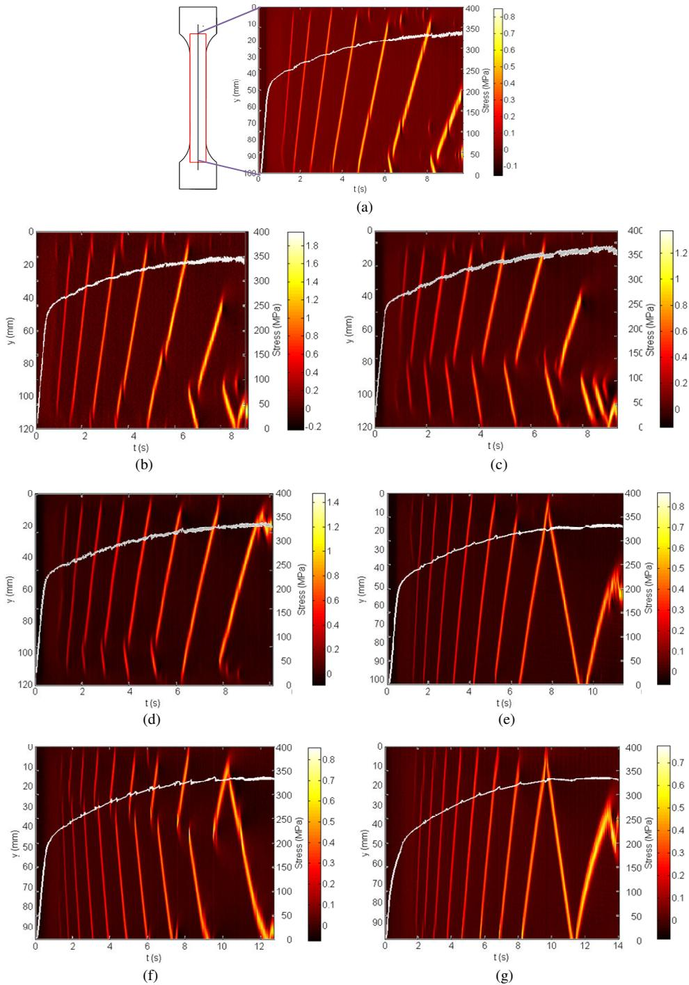
**Figure 6.** Temperature change versus time as measured by thermography along vertical center line of specimens, with stress-time curve superposed. Nominal strain rate is  $10^{-2} \text{ s}^{-1}$  and geometry is a smooth flat specimen with 15 mm width. The thickness  $e$  is (a) 1 mm, (b) 2 mm, (c) 3 mm, (d) 4 mm, (e) 5 mm, (f) 7 mm, and (g) 9 mm.
