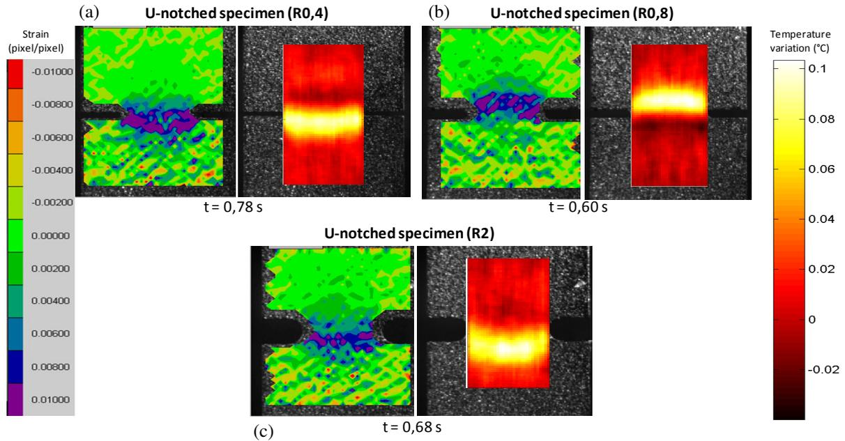
**Figure 14.** Longitudinal strain and temperature change  $\Delta T$  maps as obtained from DIC and DIT on the two opposite sides of each specimen for tests on notched specimens: (a) T1, (b) T2, and (c) T3.
