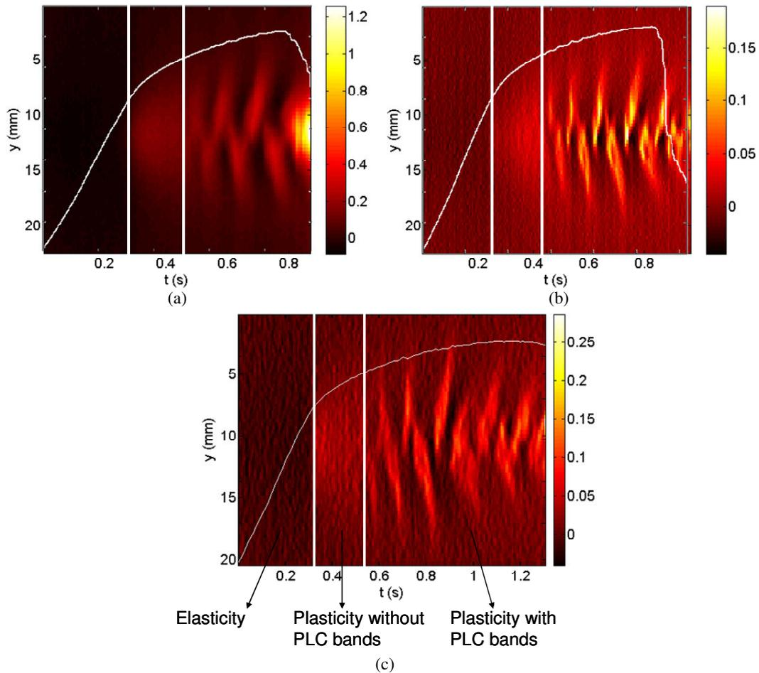
**Figure 11.** Temperature change  $\Delta T(4.84, y, t)$  measured along the vertical line  $x = 4.84$ , in comparison with the response force-time of the test. Note clearly the elasticity, the plasticity without PLC bands, and the plasticity with PLC bands for the three tests: (a) T1, (b) T2, and (c) T3.
