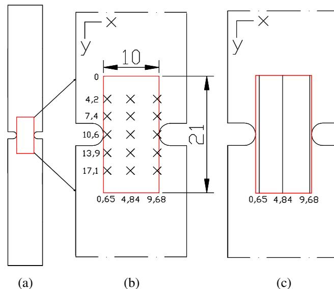
**Figure 1.** (a) Flat U-notched specimen with a 2 mm radius notch (T3) used in the investigation showing the imaged zone area for digital infrared thermography (DIT); (b, c) zooms of the imaged area indicating the locations used for presenting some of the experimental results in Section 3.2.
