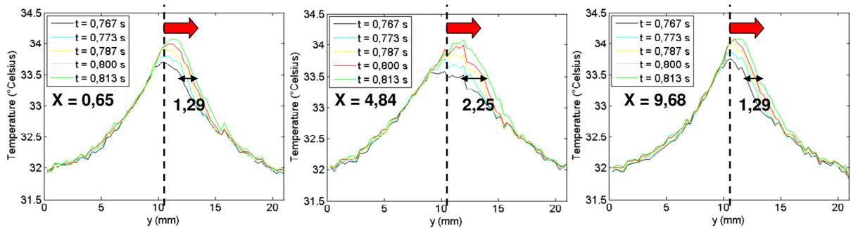
**Figure 19.** Propagation of band 2 shown in Figure 15. The travel distance of the band is higher in the minimal section ( $x = 4.84$ ) than at the roots of the notches ( $x = 0.65$  and  $x = 9.68$ ) leading to the slightly curved morphology of the band.
