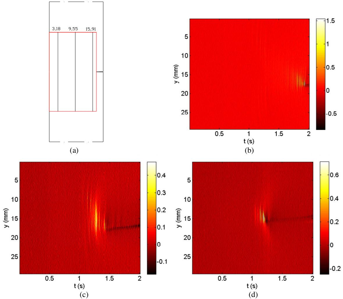
**Figure 12.** (a) Cracked specimen with the imaged area indicating the three vertical lines used for presenting the experimental results; (b) temperature change  $\Delta T(x, y, t)$  measured along the vertical line  $x = 3.18$ ; (c) temperature change  $\Delta T(x, y, t)$  measured along the vertical line  $x = 9.55$ ; (d) temperature change  $\Delta T(x, y, t)$  measured along the vertical line  $x = 15.91$ .
