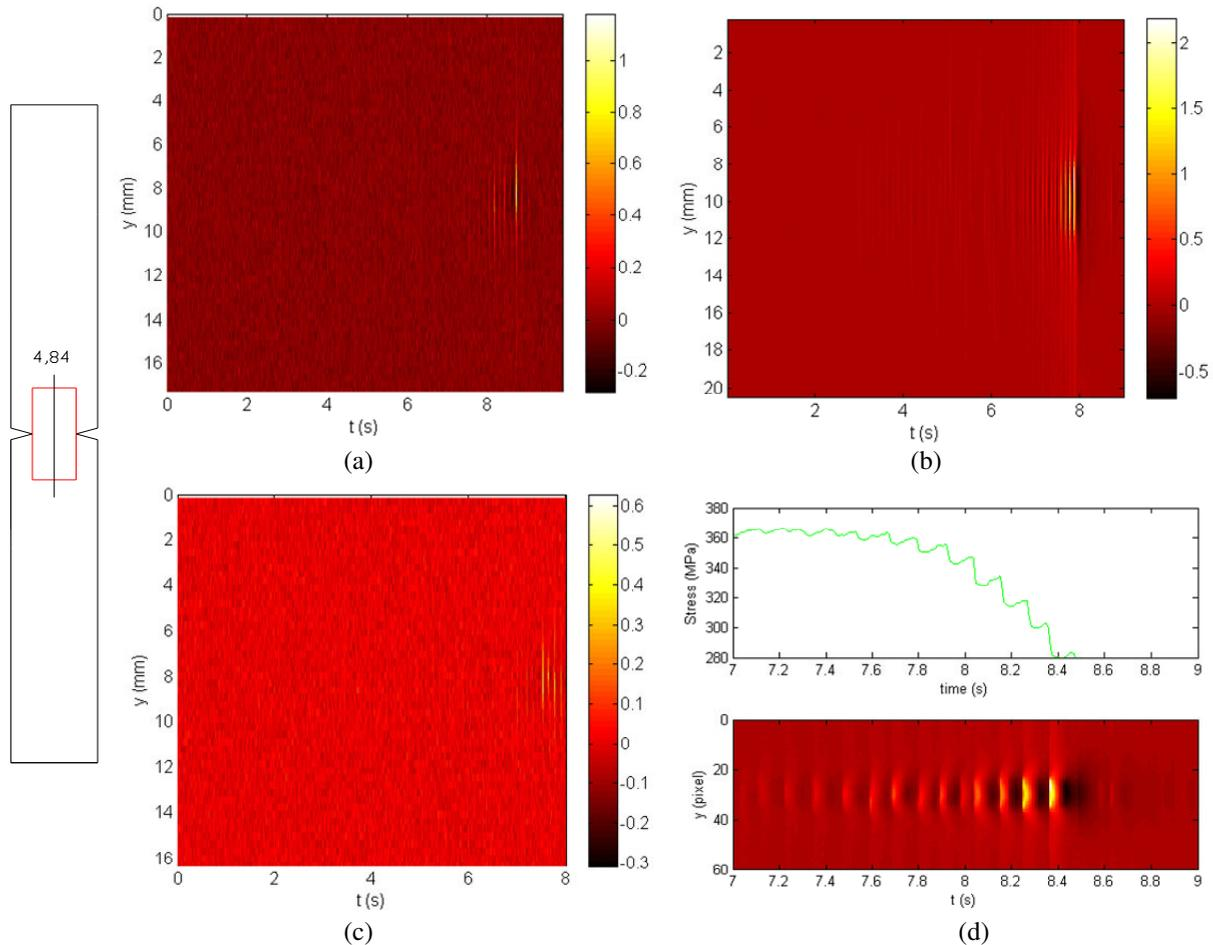
**Figure 13.** Temperature change  $\Delta T(x, y, t)$  measured along the vertical line  $x = 4.84$  for the V-notched specimens: (a) T5 (30°), (b) T6 (45°), (c) T7 (60°), and (d) T6 (V45°), showing its comparison with the response force-time at the end of the test.
