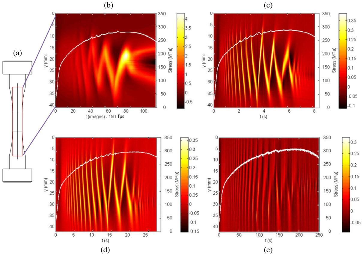
**Figure 4.** Temperature change  $\Delta T$  given by (1) versus time as measured by thermography along the vertical center line of the specimens. For completeness, the stress-time curve is superposed. (a) Round specimen ( $\phi = 6$  mm) with the imaged zone indicated; (b)  $\dot{\epsilon} = 10^{-1} \text{ s}^{-1}$ ; (c)  $\dot{\epsilon} = 10^{-2} \text{ s}^{-1}$ ; (d)  $\dot{\epsilon} = 2.8 \times 10^{-3} \text{ s}^{-1}$ ; (e)  $\dot{\epsilon} = 3.33 \times 10^{-4} \text{ s}^{-1}$ .
