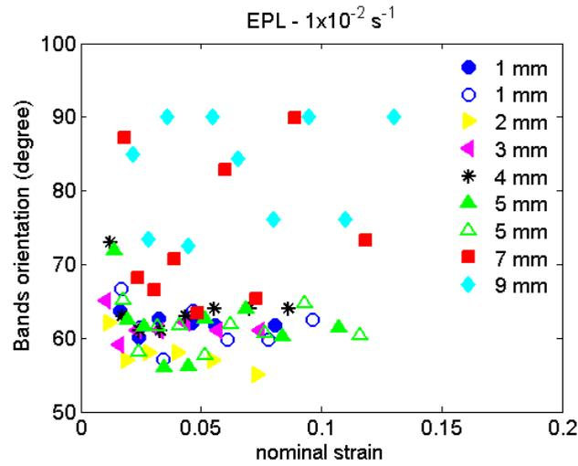
**Figure 7.** Band orientation versus nominal strain obtained during tension tests on different smooth flat specimens with the same 15 mm width but different thicknesses (1, 2, 3, 4, 5, 7, and 9 mm), at a nominal strain-rate of  $10^{-2} \text{ s}^{-1}$ .
