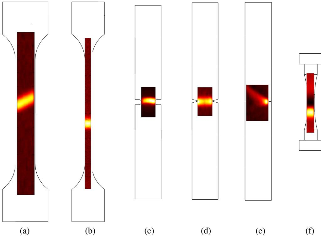
**Figure 8.** Two-dimensional view of PLC bands for different specimen geometries measured by thermography during tensile tests: (a) flat specimen, (b) prismatic specimen, (c) U-notched specimen, (d) V-notched specimen, (e) cracked specimen, and (f) round specimen. The temperature change  $\Delta T$  given by (1) is displayed here.
