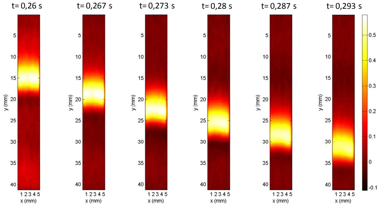
**Figure 3.** Sequence of six DIT images showing the propagation of a PLC deformation band during a tension test in a round specimen ( $\phi = 6$  mm) with nominal strain rate  $10^{-1} \text{ s}^{-1}$ . The figure displays only the imaged zone of the specimen. The temperature increment  $\Delta T$  given by (1) is displayed here.
