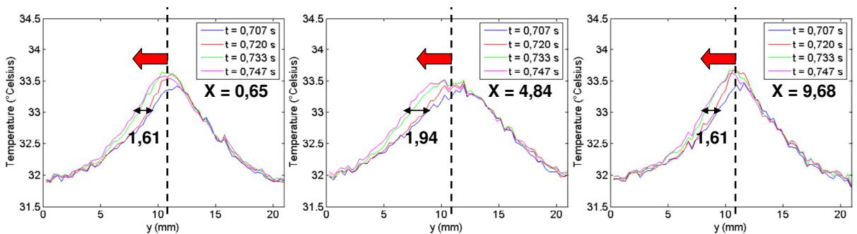
**Figure 18.** Propagation of band 1 shown in Figure 15. The traveling distance of the band is higher in the minimal section ( $x = 4.84$ ) than at the roots of the notches ( $x = 0.65$  and  $x = 9.68$ ) leading to the slightly curved morphology of the band.
