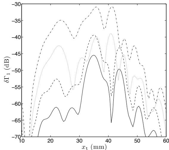
**Figure 2.** Signal response ( $\delta\Gamma_1$ ) as a function of the position ( $x_t$ ) of a 2 MHz transmitter for different sizes of the crack,  $2 \times 2$  mm (solid),  $2 \times 4$  mm (dashed),  $3 \times 3$  mm (dotted), and  $3 \times 6$  mm (dash-dotted).
