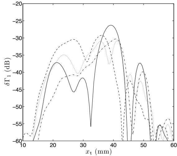
**Figure 5.** Signal response ( $\delta\Gamma_1$ ) as a function of the position ( $x_t$ ) of a 2 MHz transmitter for various values of the orientation of the crack,  $\varphi = 0^\circ$  (horizontal crack, solid),  $\varphi = 45^\circ$  (dashed),  $\varphi = 90^\circ$  (vertical crack, dotted),  $\varphi = 135^\circ$  (dash-dotted).
