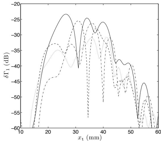
**Figure 4.** Signal response ( $\delta\Gamma_1$ ) as a function of the position ( $x_t$ ) of a 2 MHz transmitter for various values of the position of the crack relative to the corrugated interface,  $a_c = 1.25$  mm (solid),  $a_c = 2.5$  mm (dashed),  $a_c = 3.75$  mm (dotted),  $a_c = 0$  (dash-dotted).
