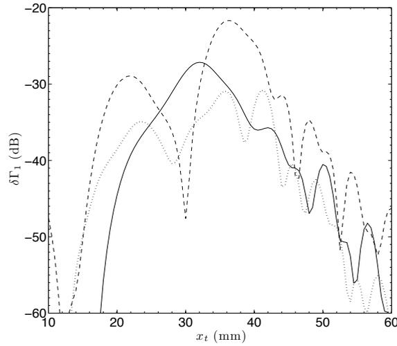
**Figure 3.** Signal response ( $\delta\Gamma_1$ ) as a function of the position ( $x_t$ ) of a 2 MHz transmitter for various values of the amplitude of the interface,  $b = 0$  (solid),  $b = 0.5$  mm (dashed),  $b = 1$  mm (dotted).
