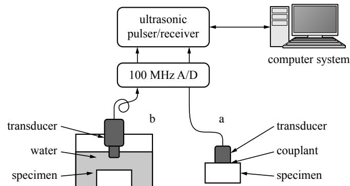
**Figure 2.** Schematic of the experimental setup: (a) contact method and (b) immersion method.
