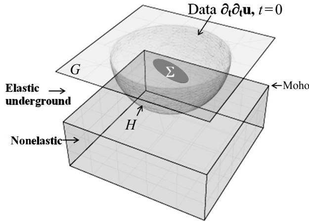
**Figure 1.** The seismic model. Part time measurement of the acceleration on the stress-free ground  $G$ , inside a circular area of radius  $c_p T$  during the time  $T$ ;  $H$  is a hemispherical surface tangent to the Mohorovičić discontinuity containing a small fault  $\Sigma$  near the ground. All seismic signals are inside the elastic hemisphere, for  $0 < t < T$ .
