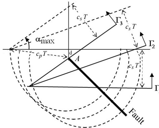
**Figure 3.** Adjoint S-waves propagating upwards. The angles between the propagating vectors and the vertical depend on the depth  $d$  of the nearest point  $A$  to the ground. The maximum angle is for the front  $\Gamma_3$ , the minimum (zero value) for the front  $\Gamma_1$ .
