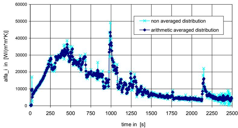
**Figure 9.** Solution to the inverse problem for real measurement. The thermocouples were placed at  $s_1 = 8 \text{ mm}$  and  $s_2 = 57 \text{ mm}$  from the inner surface.
