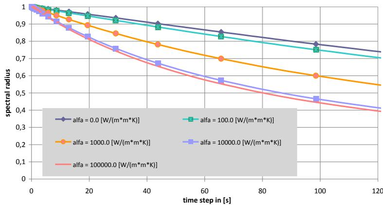
**Figure 4.** Influence of time step on the spectral radius of the stability matrix of the inverse problem ( $\zeta = 0.75$ ) for given values of heat transfer coefficient at the outer surface.
