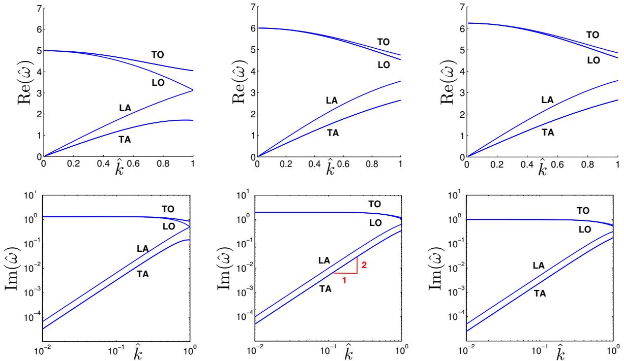
**Figure 3.** Dispersion characteristics (top row) and damping characteristics (bottom row). Left: BCC lattice with  $\zeta = 0.05$ . Middle: FCC lattice with  $\zeta = 0.05$ . Right: FCC lattice with  $\zeta = 0.025$ . In all cases  $r_K = 1$ ;  $r_D = 1$ .
