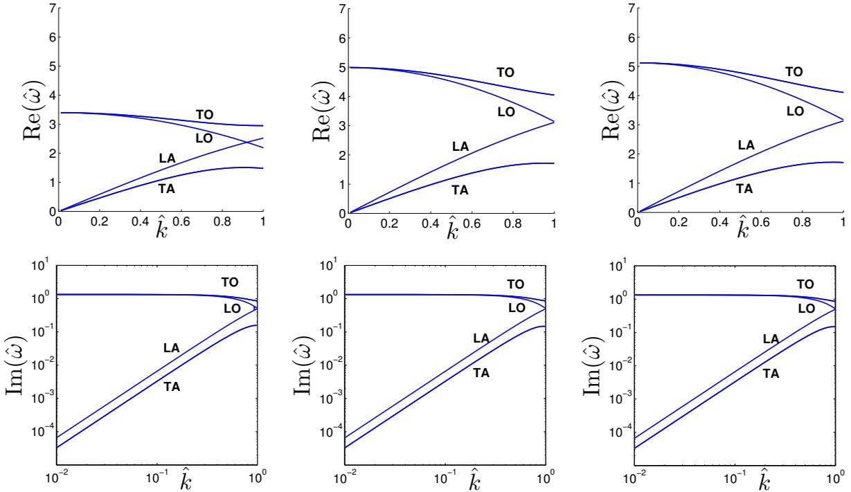
**Figure 4.** Dispersion characteristics (top row) and damping characteristics (bottom row). Left:  $r_K = 0.5$ ,  $r_D = 1$ . Middle:  $r_K = 1$ ,  $r_D = 1$ . Right:  $r_K = 1$ ,  $r_D = 0.5$ . In all cases the BCC lattice is considered, with  $\zeta = 0.05$ .
