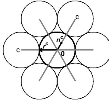
**Figure 1.** Example of a two-dimensional lattice with coordination number  $Z = 6$ . Also indicated are the contact normal vector  $\mathbf{n}^c$  and the vector  $\mathbf{r}^c$  from the center of the particle to the point of contact.
