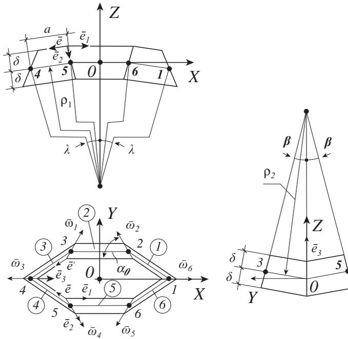
**Figure 4.** Sizes of the six-link loop cell.
