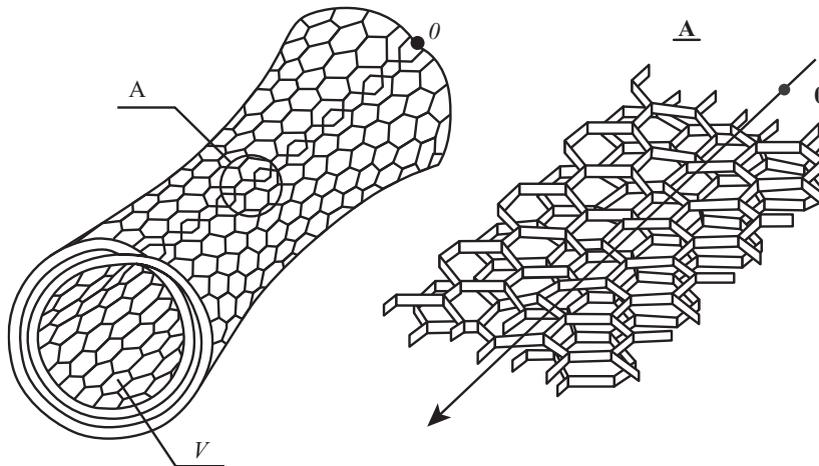
**Figure 11.** Reduction in internal volume when the shell is deployed. On the right, the arrow indicates the intersection line arising at deployment. The volume  $V$  within the surface reduces when the shell deploys.
