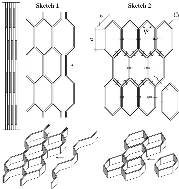
**Figure 1.** Net of rectangles connected with cylindrical hinges.
