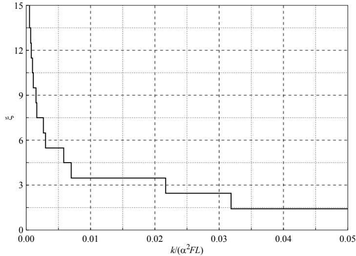
**Figure 7.** Values for the parameter  $\xi$  as a function of the connection spring stiffness  $k$  normalized by  $\alpha^2 FL$ , as computed from the stationarity of the TPE of equation (3-32) for the case  $\beta = \frac{1}{2}$ .
