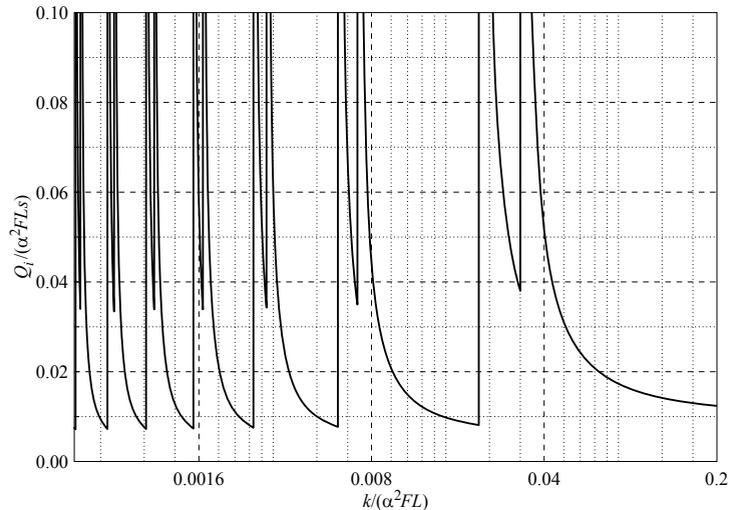
**Figure 8.** Values of the unit thrust  $Q_i$ , normalized by  $\alpha^2 FLs$ , as a function of the normalized spring stiffness  $k/\alpha^2 FL$ , for  $\beta = \frac{1}{2}$  and  $\xi$  as in Figure 7, as given by (3-29). Other data are: rectangular cross-section  $5 \times 50$  mm,  $E = 210000$  MPa,  $L = 560$  mm,  $s = 0.5$  mm,  $\Delta = 11.2$  mm.
