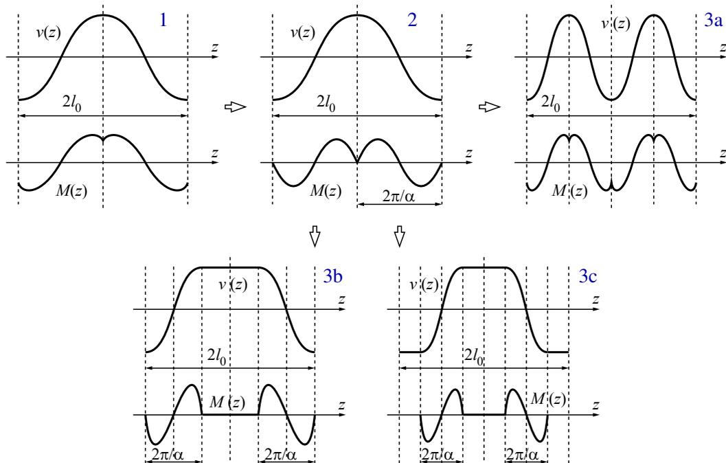
**Figure 3.** Possible evolution of the buckled shape after the first contact. One or two buckled waves are depicted. Image 2 refers to the instant when both the inclined portions of the beam reach a critical axial load value, with zero bending moment at the contact point. Images 3a, 3b, and 3c illustrate possible evolutions from the situation of image 2.
