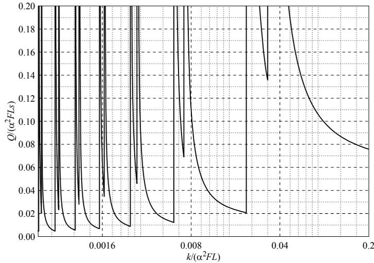
**Figure 9.** Values of the total thrust  $Q$ , normalized by  $\alpha^2 FL_s$ , as a function of the normalized spring stiffness  $k/\alpha^2 FL$ , for  $\beta = \frac{1}{2}$  and  $\xi$  as in Figure 7, as given by (3-4) and (3-5). Other data as in Figure 8.
