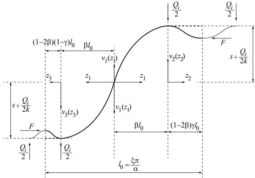
**Figure 6.** Structural scheme of a single half-wave of the buckled deformed shape. The solid lines represent a generic configuration of point contact. The dashed lines represent a generic configuration of line contact. Parameters  $\xi$ ,  $\beta$ , and  $\gamma$  are unknown and define the geometrical properties of the half-wavelength  $l_0$ .
