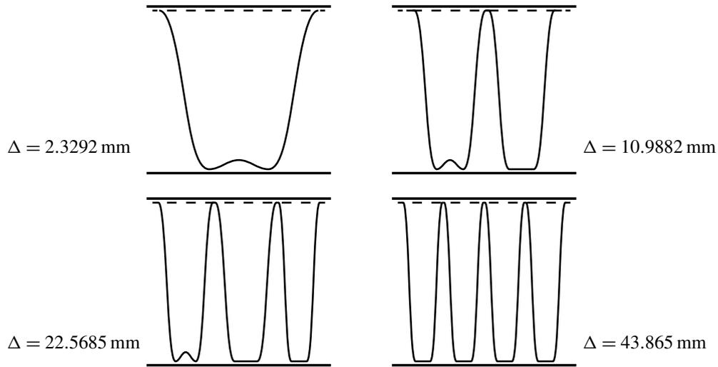
**Figure 2.** Deformed shape, magnified by a factor of 100, at four axial displacement values for a beam problem adopting the data of Figure 5 of [Chai 1998]. Dashed lines indicate undeformed shapes; thick solid lines indicate the final position of the rigid containment surfaces. FEM solution; 500 Timoshenko linear beam elements. Data as noted in the text.
