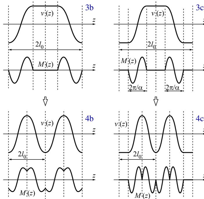
**Figure 4.** Possible evolution of the buckled shape from line contact situations. Images 3b and 4b refer to the evolution from an ALC configuration, and images 3c and 4c to the evolution from an SLC configuration.
