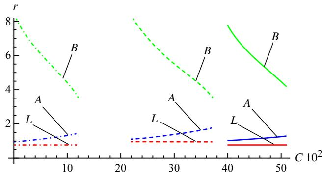
**Figure 12.** Equilibrium positions of the crack tips depending on relative cohesion  $C$  for various  $k$ : solid lines correspond to  $k = 0$ ; dashed lines correspond to  $k = 0.1$ ; dash-dotted lines correspond to  $k = 0.33$ .
