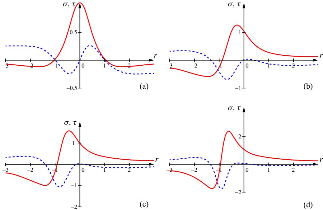
**Figure 3.** Profiles of dimensionless stresses caused by the wedge on the interface inclined at (a)  $\theta = \pi/2$ , (b)  $\theta = \pi/3$ , (c)  $\theta = \pi/4$ , (d)  $\theta = \pi/6$  for Configuration 2 as functions of the parameter  $\rho$ ; solid lines are normal stresses, dashed lines are shear stresses.
