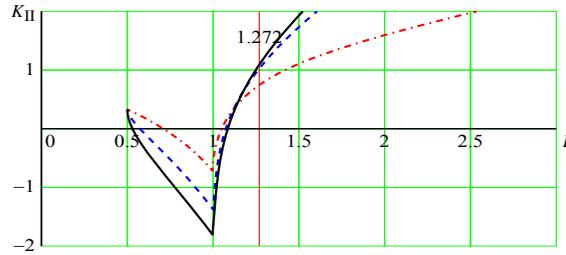
**Figure 10.** Dependence of dimensionless  $K_{II}$  on  $L$  for various combinations of the friction angles and cohesion for  $L_0 = 0.5$ ; dash-dotted line corresponds to  $\rho = 0^\circ$ , dashed line corresponds to  $\rho = 15^\circ$ , solid line corresponds to  $\rho = 30^\circ$ .
