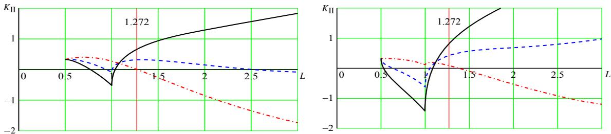
**Figure 9.** Dependence of dimensionless  $K_{II}$  on  $L$  for various values of the friction angle (left) and the cohesion (right), for  $L_0 = 0.5$  and  $C = 0$ ; dash-dotted line corresponds to  $\rho = 0^\circ$ , dashed line to  $\rho = 15^\circ$ , solid line to  $\rho = 30^\circ$ .
