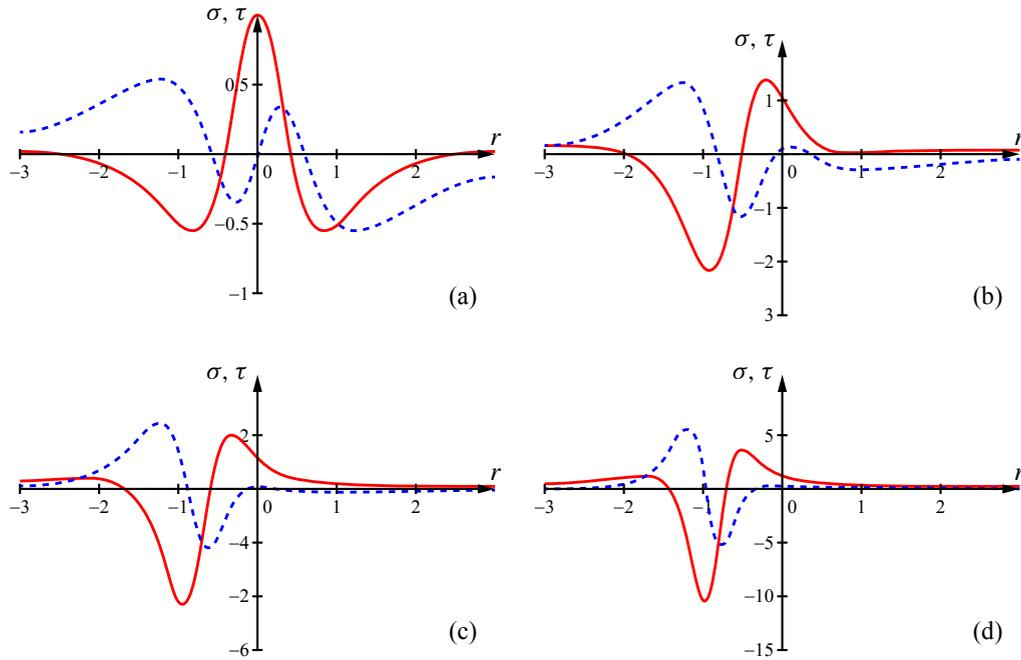
**Figure 2.** Profiles of dimensionless stresses caused by the wedge on the interface inclined at (a)  $\theta = \pi/2$ , (b)  $\theta = \pi/3$ , (c)  $\theta = \pi/4$ , (d)  $\theta = \pi/6$  for Configuration 1 as functions of the parameter  $\rho$ ; solid lines are normal stresses, dashed lines are shear stresses.
