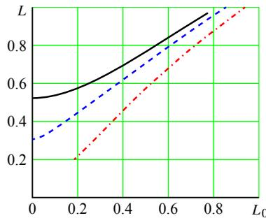
**Figure 11.** The half-length of the sliding zone  $L$  as a function of the half-length of the delamination zone  $L_0$  for various cohesions at  $k = \tan 30^\circ$ ; dash-dotted line corresponds to  $C = 0.5$ , dashed line corresponds to  $C = 0.1$ , solid line corresponds to  $C = 0.5$ .
