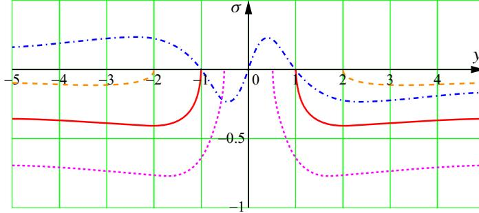
**Figure 4.** The stresses on the interface after delamination for  $L_0 = 0.5, 1, 2$ ; dots are normal stress for  $L_0 = 0.5$ , solid line is normal stress for  $L_0 = 1$ , dashed line is normal stress for  $L_0 = 2$ , dash-dotted line is shear stress.
