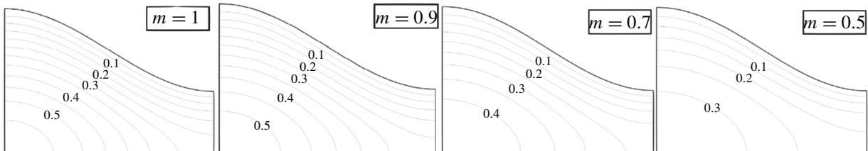
**Figure 6.** Equivalocity lines for different values of power-law index  $m$ .
