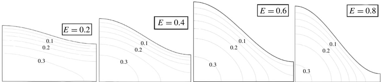
**Figure 5.** Equivalocity lines for different values of corrugation amplitude.
