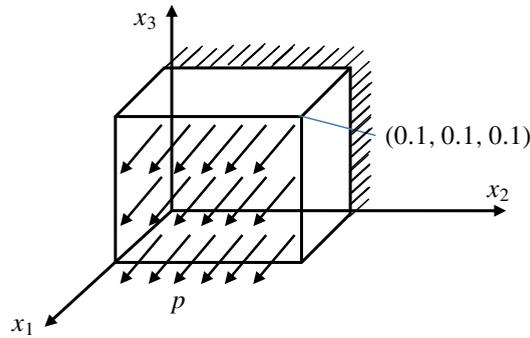
**Figure 1.** Loads and boundary conditions of considered body.
